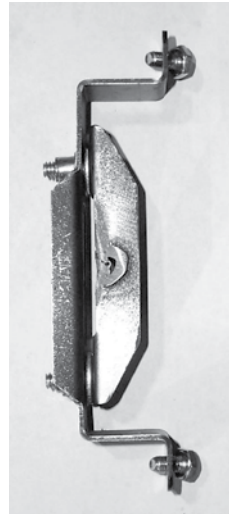
Latch Assembly re-assembled with Spacers removed.
