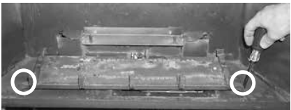
Remove the 2 screws, push Burner Assembly to the left and lift out.
