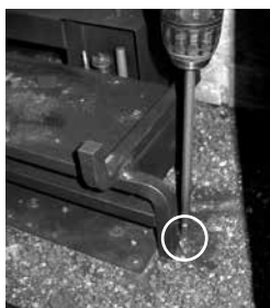
Diagram 1: Remove the left and right screws.
