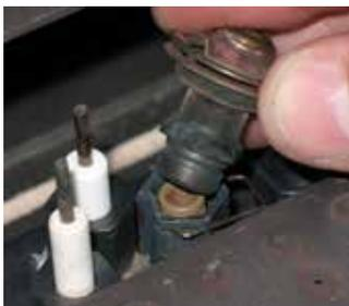
15. Unscrew the pilot orifice with the Allen key; then replace with the LPG pilot orifice and the pilot cap, provided in the kit.
