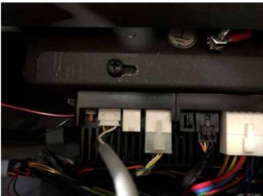
5. Locate the dongle holder on the right side of the IFC.
