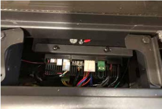
3. Locate the WIFI dongle connection (X0A) on the left side of the IFC.
