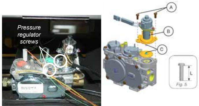
9. Re-attach the Pressure Regulator wire (disconnected in Step 6), and resituate the IFC, secure the screws that fasten the IFC Mounting Brackets.
