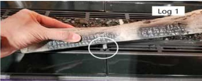
7. Lay the log on the firebox. Ensure the bottom left end of the log is 7/8" away from the edge of the firebox.
