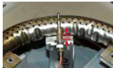
Schéma 4 - correct thermocouple position
