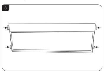
3.3 The fireplace can now be positioned in the opening. Level the appliance, and attach the unit to the frame using the fixing holes provided, see Diagram 4.
