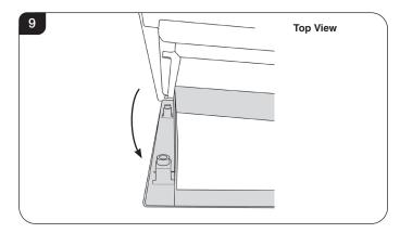
4.3 There is a clamp at the top of each corner of the glass viewing panel that secure the glass in place, see Diagram 10.
