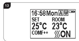
If the heater is on in the current period, pressing the button will turn the heater off.
