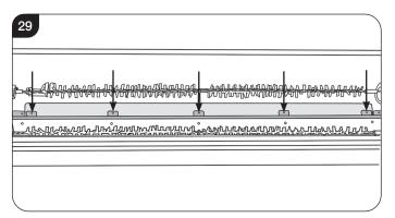
NOTE: When refitting the shield ensure that the lip curves down and towards the back. It will be necessary to lift the shield slightly to align the screws. Refit the screws from inside out.
