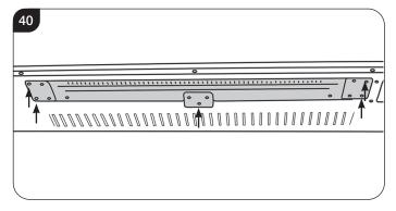
16.4 Carefully lower the Heater Assembly. This will require a slight tipping motion to clear the edge, see Diagram 41. NOTE: The Heater Assembly has wires attached.
