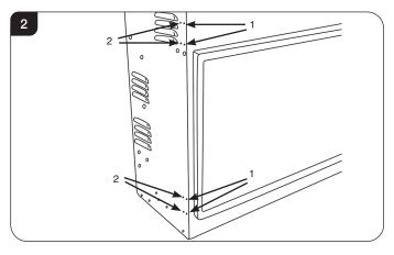
3.2 Attach the 4 fixing brackets to the sides of the appliance, see Diagram 3.
