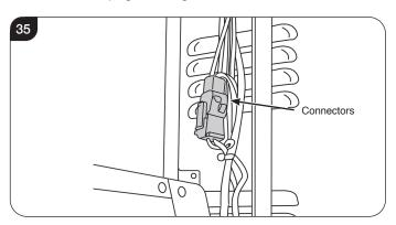
14.5 Replace in reverse order, ensuring the cable ties are replaced.
