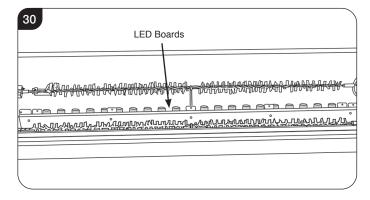
12.4 The LED boards are coupled together at the end of each board and held in place by clips, see Diagram 31.
