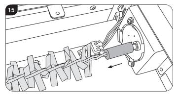
7.5 Withdraw the spindle from the left hand bracket, see Diagram 16.
