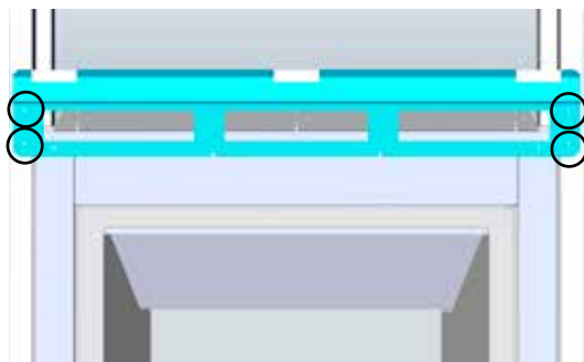
Diagram 3 -Bracket screw locations.
