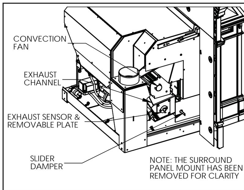
Figure 15: Slider/Damper Plate & Rod in Unit.
