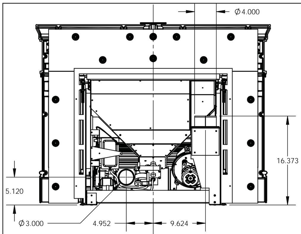
Figure 8: GCI60 Inlet and Outlet Location.
