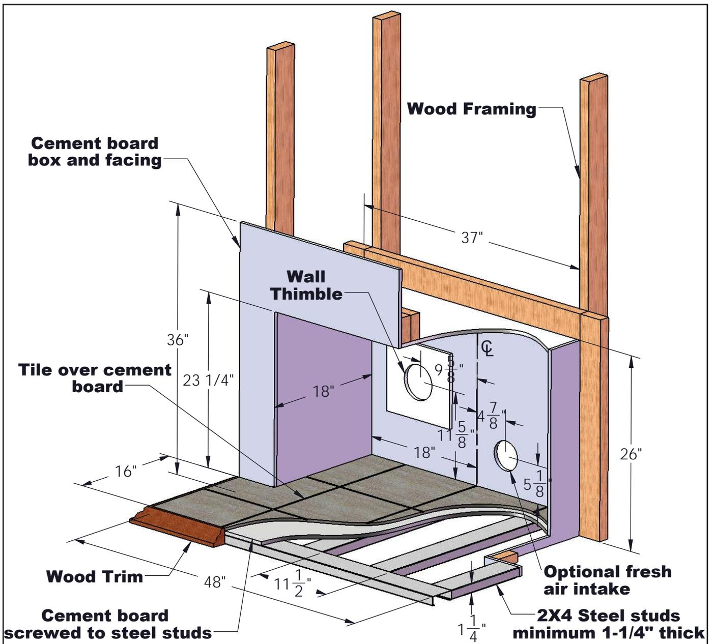
Figure 11: Built-In Specifications
