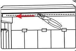
5. To reinstall or replace, first slide left side of tube into hole on left side air channel. Align tab on right side air channel with notch on right hand end of air tube. Firmly grip center of air tube with vise grips, use hammer to tap vise grips from left to right until the tube bottoms out into the air channel on right.
