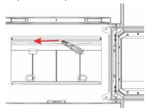
3. Install the center baffle.
