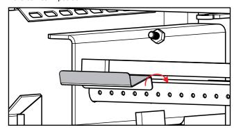
7. Slide left and right baffle cover plates on either side of baffles as shown.
