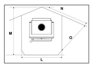
This stove may be connected to a lined masonry chimney or a listed factory built chimney suitable for use with solid fuels and conforming to ULC629 in Canada or UL-103HT in the USA. Do not connect it to a chimney serving another appliance. To do so will affect the safe operation of both appliances, and will void the stove warranty. You must comply with the local authority having jurisdiction and/or in Canada, CSA installation standard B365-M87.
