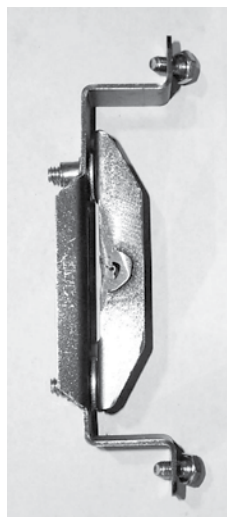
Latch Assembly reassembled with spacers removed.
