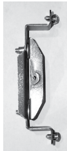
Latch Assembly reassembled with spacers removed.
