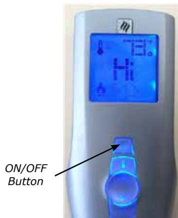
Diagram 1 Remote shown in Manual Mode on Hi
