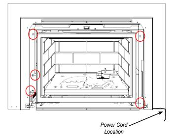
3. Route the power cord on the right side between the inner and outer profile of the faceplate. Use a grommet and wire clip to secure.
