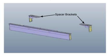
Attach the top and bottom part of the spacer brackets and then attach these spacer brackets to the assembled hearth trim with 3 screws.
