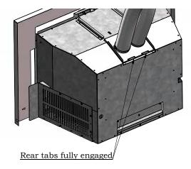
Properly installed Flue Connector Plate
