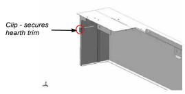
6) Line up the hearth trim with base of the unit and secure it with 3 screws as shown below.
