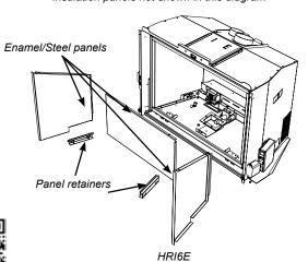
האוסב \*Insulation panels not shown in this diagram
