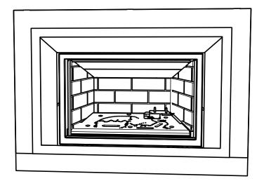
2. Install the outer faceplate by hooking the flange over the hanger as shown.
