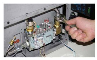
7) Remove both Screws that secure the Gas Valve Mounting brackets, both
