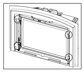
4. Install the safety screen into the inner Vignette frame by slightly tilting the safety screen frame and placing it up into the Vignette frame. Let the safety screen slightly drop down into position within the Vignette frame.
