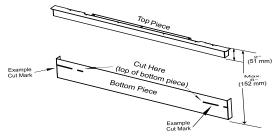
3. Reattach the top piece of the hearth trim to the cut bottom piece by fitting in place.
