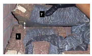
Log 7 pin locator line up with Log 1 pin
