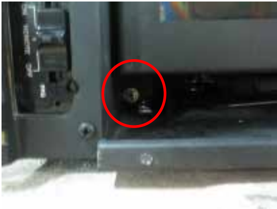
The Surefire switch is located at the bottom left corner of the unit.
