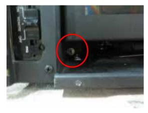
The Surefire switch is located at the bottom left corner of the unit.
