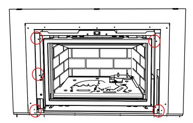
3. Separate the Outer Faceplate from the Backing Plate by removing 7 screws.
