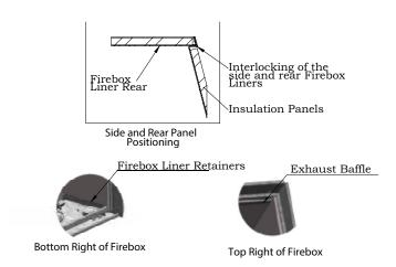
3. Install the firebox liner Left, with the corresponding Insulation Panel by sliding it into the left side of the firebox. The rear flange of the liner must fit between the firebox liner rear and the firebox. You may have to push the liner against the firebox as you push it rearward.
