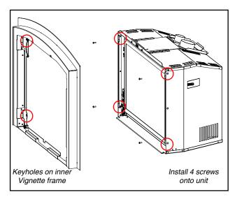
Install the inner Vignette frame by hanging the frame off the 4 screws via the keyhole openings on the frame. When in position, tighten the 4 screws.
