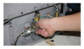
6) Disconnect the Gas Supply Line from the On/Off Safety Shut off Valve.
