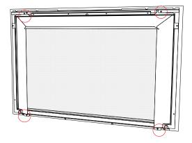
Remove 4 screws to remove safety screen assembly
