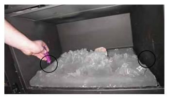
3) Lift the Burner slightly while pulling forward to clear the mixing tube.
