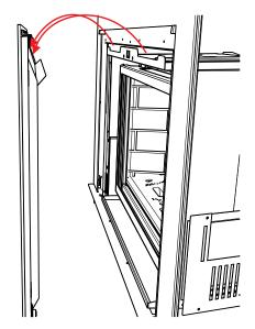
2. Remove the outer faceplate by removing the 5 screws as shown.
