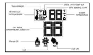
Figure 2: Transmitter LCD Display
