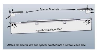
5) Secure the hearth trim with a clip on its side to keep it steady as shown in the diagram below.
