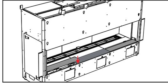
2. Slide the glass barrier stopper bracket between the front panel and the unit wall as shown.
