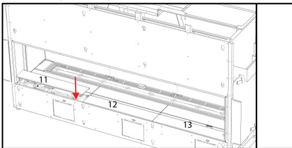
15. Slide the glass barrier stopper bracket between the front panel and the unit wall as shown.
