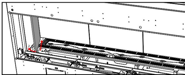
4. Secure panel in position with one screw.
