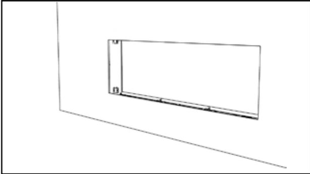
4. Hand bend attachment tabs so they bend past the magnets to the mounting bracket.
