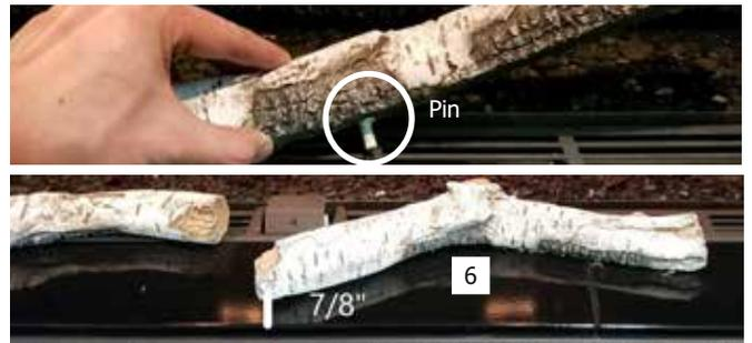
12. Insert the pin of Log 7 into the hole on the right-most side of the burner. Position the left end of Log 7 1/2" from edge of panel, as shown below.
