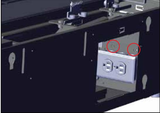
3. Slide electrical box plate towards the back of the unit and then out.
