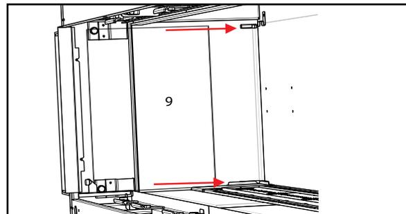
11. Secure side panel **9** with one screw on the top bracket as shown.
