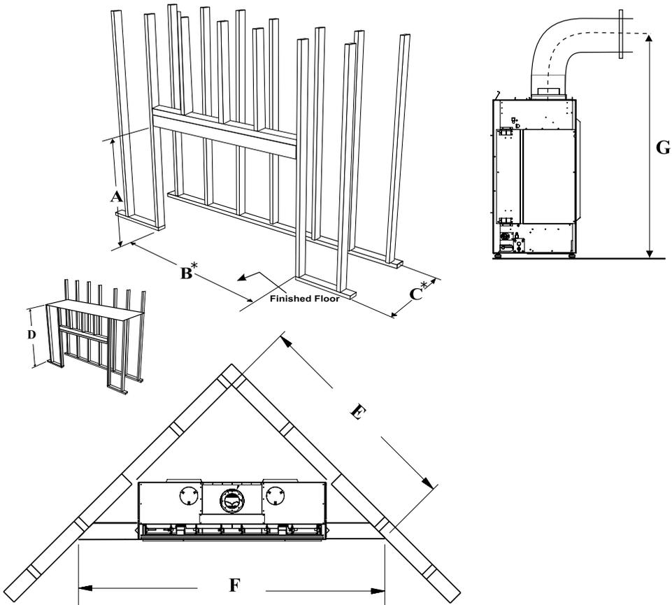
\*The framing depth/width does not take into account drywall/wood or similar materials against the back /side wall. The framing depth will need to change based on the thickness of the material.
