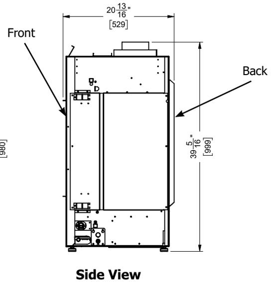
Note: Height Dimension is taken with leveling legs fully inserted and may vary depending on the height of the leveling legs, when unscrewed or extended.
