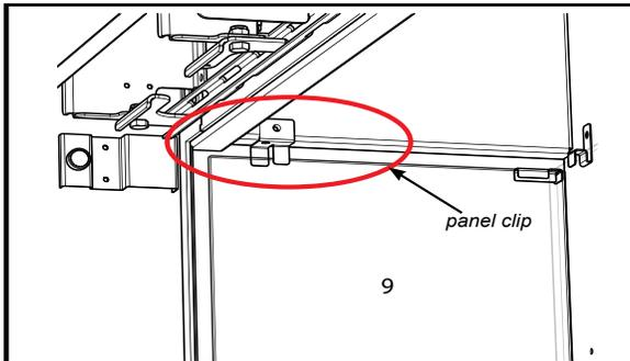
16. Install side outer panel (14) by manoeuvring the panel between the wall and the barrier stopper bracket as shown below. Repeat on other side to install panel 15. The panels are held in place by magnets.
