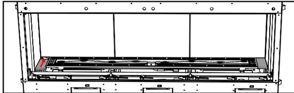
3. Slide the panel into the unit until it slips behind the back panel, then pivot it to the side of the firebox.
