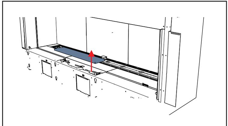
2. From inside the unit—push in tab to release the access panel at the top.
