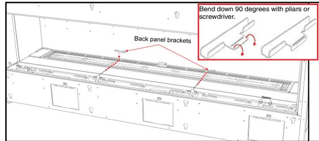
7. Carefully manoeuvre the back glass panels (6, 7, 8) to the back wall of the firebox. Start with back panel 6 -- place two panel brackets on each panel and manoeuvre into position, sliding the bottom into the corner and back brackets.
