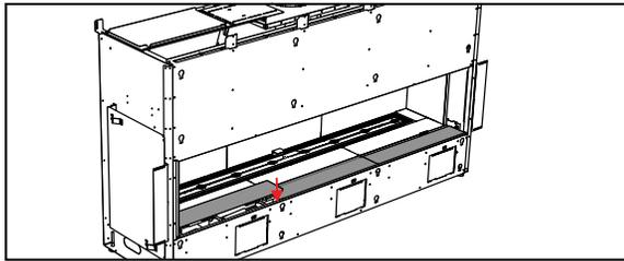
8. Slide the glass barrier stopper bracket between the front panel and the unit wall as shown.
