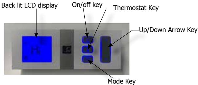
Figure 2: Proflame Transmitter
