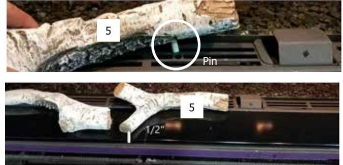
11. Insert the pin of Log 6 into the hole on the right side of the pilot. Position the left end of Log 6 7/8" from the edge of the panel.
