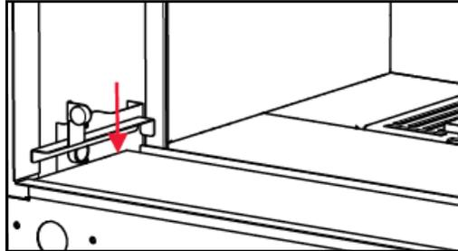
3. Install side outer panels by manoeuvring the panel between the wall and the barrier stopper bracket as shown below. The panels are held in place by magnets.
