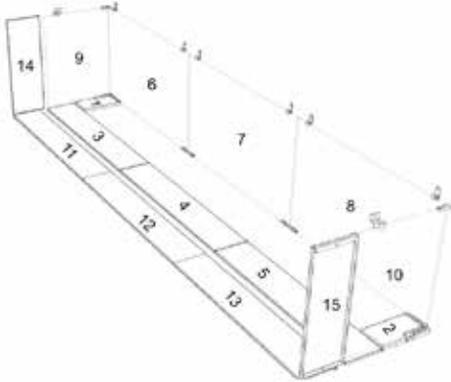
3. Install back corner panels (1, 2) - seat smallest panel in back left corner, repeat on other side.
