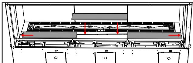
1. Install 3 front outer panels as shown below.
