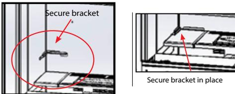
5. Install the 3 front panels (3, 4, 5) into the front firebox panel.
