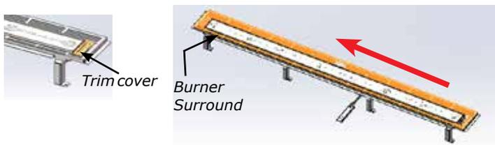
7. Remove 8 screws in locations shown below (4 at front and 4 at rear)—slide burner to the left away from the orifice and lift out.
