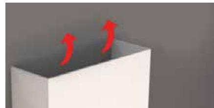
The ventilation opening may be placed on top ensuring it meets the 180 square inch opening. This type of ventilation opening would be used when the top of the enclosure is visible from above and where the ceiling within the room is higher than normal.
