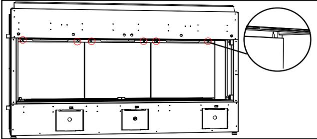
2. Slide bottom side inner panels under the back panels.
