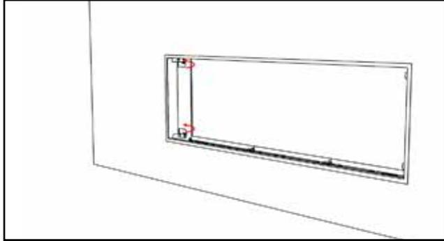
2. Prior to installing outer liner panels and barrier glass, remove finishing trim plates from right and left sides.
