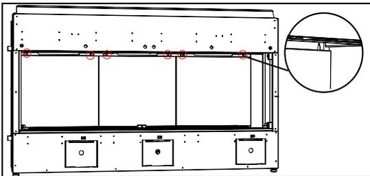
2. Slide bottom side inner panels under the back panels.
