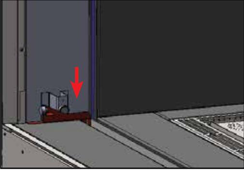
2. Slide backwall outer panel behind glass stopper bracket.
