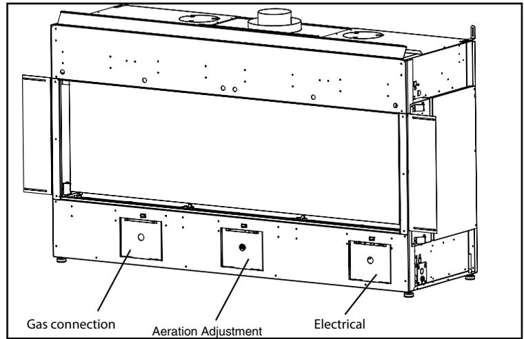
1. Identify access panel to be removed, remove corresponding outer trim panel by lifting up and off (centre panel shown below).
