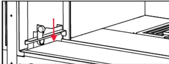
9. Install side outer panels by manoeuvring the bracket between the wall and the barrier stopper bracket as shown below. The panels are held in place by magnets.
