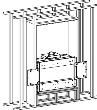
2. Locate mounting holes in locations shown below and remove nailing strips (if already installed).
