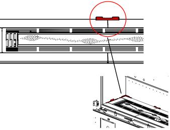
6. Slide the three #4 rear glass panels into the bottom rear and corner brackets.
