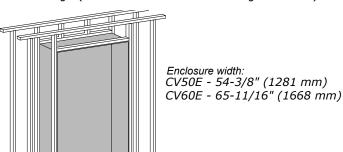
4. Move unit into framed opening at desired height and level unit on all sides. Connect gas and electrical (see manual).
