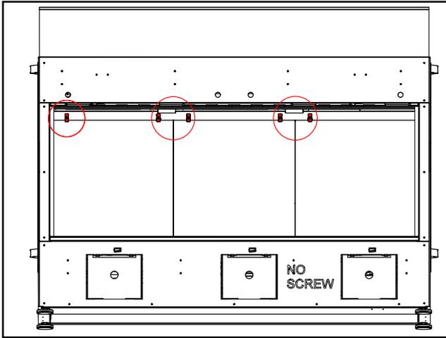
8. Slide the side glass panel #5 into the bottom side bracket and secure the side glass by mounting the top bracket and tightening the 2 screws. Do for both sides.
