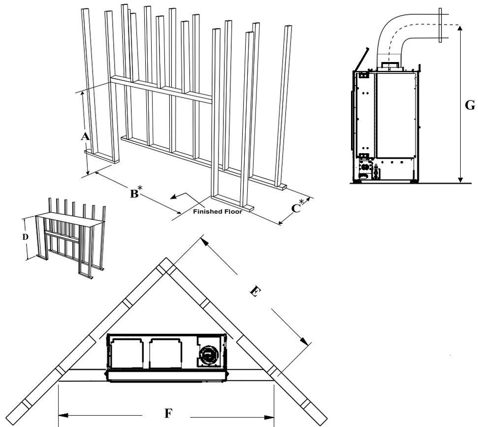
Note: This appliance must be installed on a solid surface such as a plywood floor which must be the full width and depth of the appliance.
