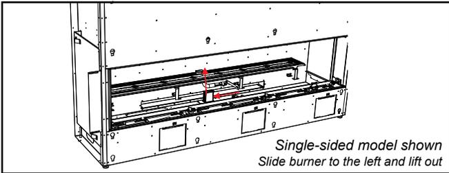
13. Remove burner orifice with a 3/8" wrench. Use another wrench to hold on to the elbow behind the orifice. Discard orifice. Reinstall new burner orifice LPG stamped #52 and tighten.
