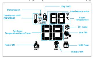
Figure 1: Transmitter LCD Display
