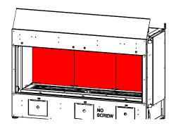
7. Secure the rear glass by mounting top bracket as shown below.
