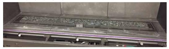
6. Locate the hole on the burner surround, on the left side of the pilot. Insert the pin underneath Log 1 into the hole on the burner surround.
