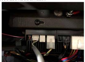
5. Locate the dongle holder on the right side of the IFC. If no dongle holder present, apply the provided Velcro strips to the dongle and stick the dongle onto the closest clamp bracket to the IFC.
