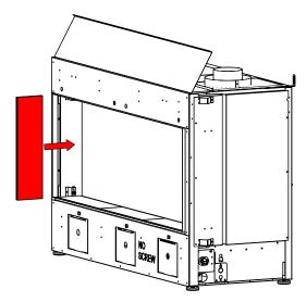
13. Clean the outer panels with a cloth before installing the safety outer barrier glass. To install the safety glass, see this manual for instructions.
