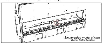
14. Remove pilot retainer clip with pliers and pull off the pilot cap to expose the pilot orifice.
