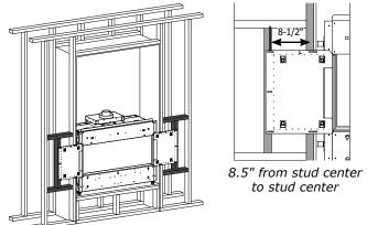
3. Attach left and right base panels using 2 screws on each side. Remove drywall finishing edge from right and left sides of window opening using supplied right-angle screwdriver. Screws only need to be loosened to remove both finishing trims. Once removed, retighten screws and discard finishing trim.
