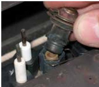
15. Unscrew the pilot orifice with the Allen key; then replace with the LPG pilot orifice and the pilot cap, provided in the kit.
