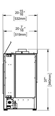
Note: Height Dimension is taken with leveling legs fully inserted and may vary depending on the height of the leveling legs, when unscrewed or extended.
