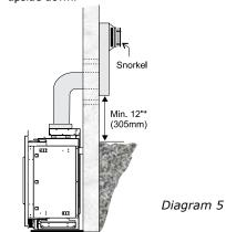
\*As specified in CSA B149.1 Installation Code. Local codes or regulations may require different clearances.
