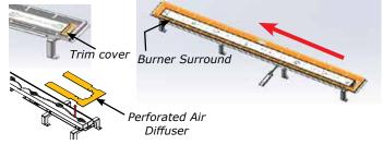
12. Loosen 8 screws in locations shown below (4 at front and 4 at rear)—slide burner to the left away from the orifice and lift out.
