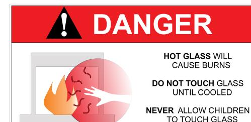
A barrier designed to reduce the risk of burns from the hot viewing glass is provided with this appliance and must be installed for the protection of children and other at risk individuals.
