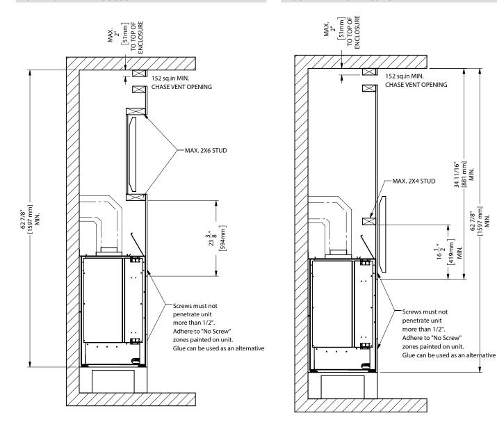
Note: The TV mounting bracket cannot be secured directly to the appliance. It must be secured to framing. The TV depicted in the picture may need to be higher depending on the style of TV mounting bracket used.
