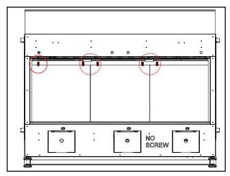
8. Slide the side glass panel #5 into the bottom side bracket and secure the side glass by mounting the top bracket and tightening the 2 screws. Do for both sides.
