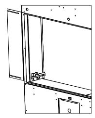
9. Slide the side #6 outer panels between the wall and the barrier stopper bracket. Repeat steps to install the remaining three #6 outer panels using a barrier stop where required.
