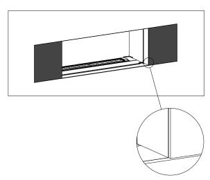
Correctly installed glass panels
