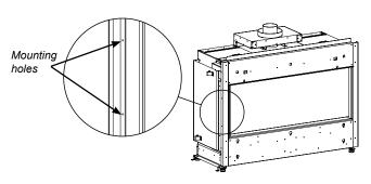
2. Locate mounting holes in locations shown below and remove nailing 5. Install a second stud as shown. The distance from first to second stud should be 8-1/2"
