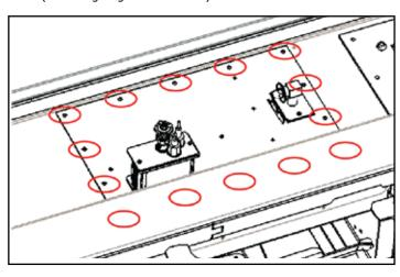
10. Lift valve tray out partially and disconnect flexible gas connection on the valve inlet side, remove valve tray- replace with new valve tray & valve assembly gasket.
