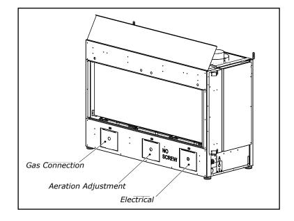
1. Identify access panel to be removed, remove corresponding outer trim panel by lifting up and off (centre panel shown below).
