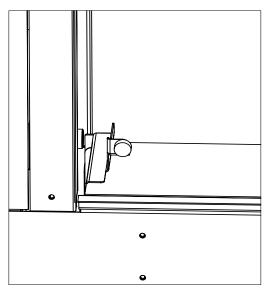
12. Slide the side outer #7 glass panels between the wall and the barrier stopper bracket. If the unit does not have a barrier stopper, stick the side outer panels to the magnets.
