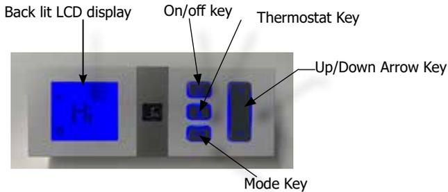
Figure 2: Proflame Transmitter
