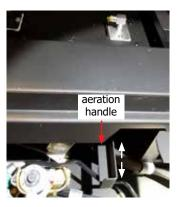
NOTE: The aeration handle is located near the right hand side of the gas valve access door -- attached by a magnet.
