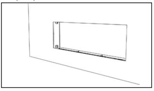
2. Prior to installing outer liner panels and barrier glass, remove finishing trim plates from right and left sides.
