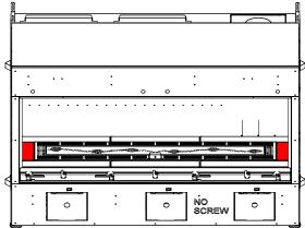
4. Install the 5 screws loosely and install the three #3 panels in the rear of the firebox.
