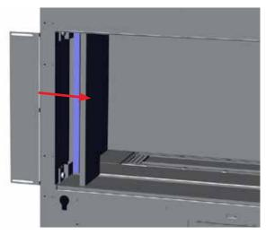
2. Slide the stopper bracket in between the front panel and the unit wall as
