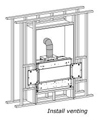
8. Finish the wall with desired finishing material and install rear enclosure venting (see manual for finishing/venting requirements).
