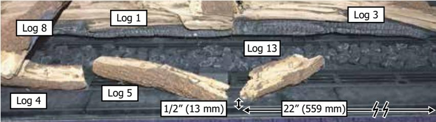
16. Place log 9 on to the pin of log 1 as shown below. Align the other end of log 9 so it is touching off on log 5 and 13 as shown below.
