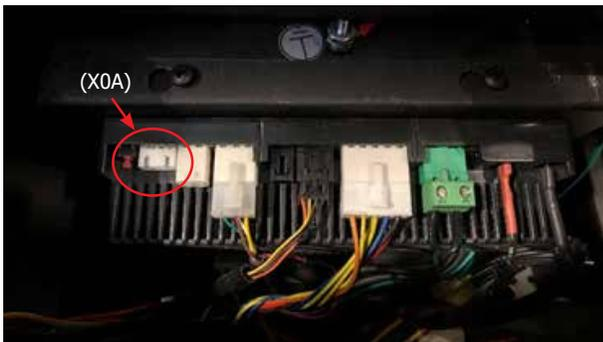
4. Line up the tabs on the dongle with the notches on the IFC connection and insert the cable into the connection.
