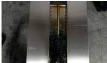
1. Start pouring Crystals on one end of the burner.
