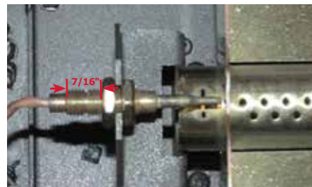
Diagram 4 Correct thermocouple placement
