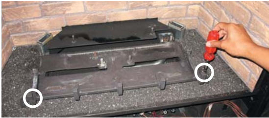
Diagram 1: Remove the left and right screws.
