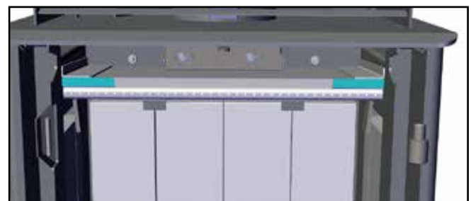
Baffle brackets and cover plates in final position
