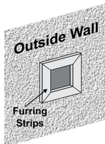
**Note:** If installing termination on a siding covered wall, furring strips must be used to ensure that the termination is not recessed into the siding.
