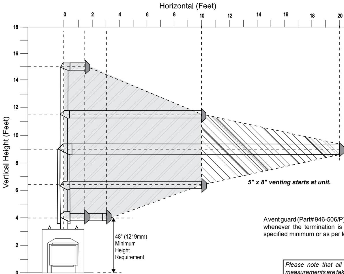
A vent guard (Part# 946-506/P) should be used whenever the termination is lower than the specified minimum or as per local codes.
