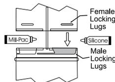
**NOTE:** For best results and optimum performance with each approved venting system, it is highly recommended to apply "Mill-Pac" sealant (supplied) to every inner pipe connection. Failure to do so may result in drafting or performance issues not covered under warranty. Silicone (red RTV) is optional.
