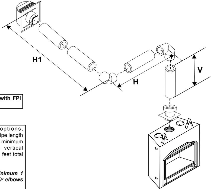
**Must Use: 5" x 8" Simpson Direct Vent Piping with FPI Inverter Starter Collar (Part #946-605).**
