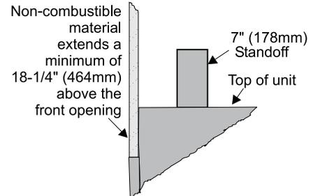
**Install Top Standoffs & Side Nailing Strips before unit is slipped into position. See the "Unit Assembly Prior to Installation" section for assembly details.**
