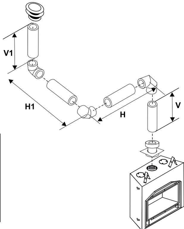
**Must Use: 5" x 8" Simpson Direct Vent Piping with FPI Inverter Starter Collar (Part #946-605).**
