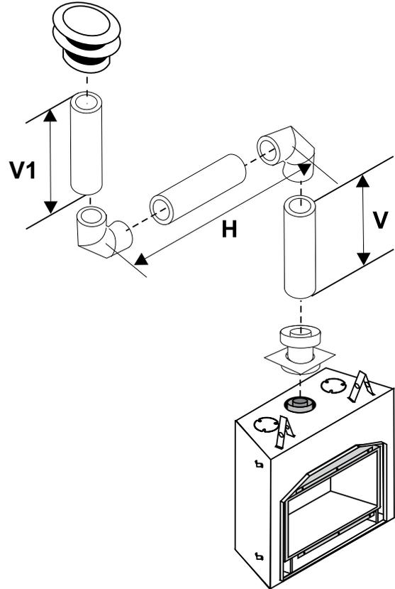
**Must Use: 5" x 8" Simpson Direct Vent Piping with FPI Inverter Starter Collar (Part #946-605), unless V1 is greater than or equal to 4'-6" then use 4" x 6-5/8" piping.**
