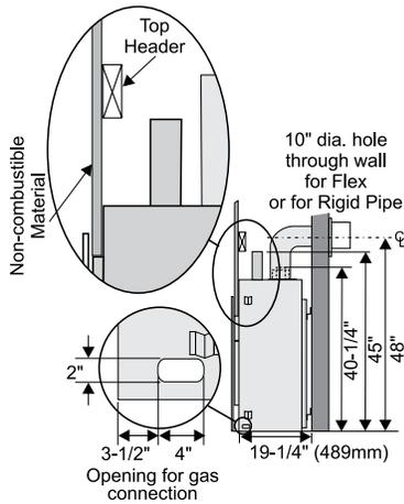
**Heat Wave** The *HeatWave* Duct Kit has different clearance and framing requirements, check the *HeatWave* manual for details.
