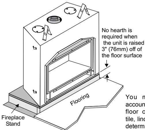
You must take into account the depth of the floor covering (carpet, tile, linoleum, etc.) when determining the height of the fireplace stand.
