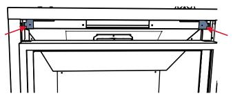
Install the heat deflector with three (3) screws - the screws are located on under the top of the unit. Loosen the screws-slide deflector on and tighten screws.
