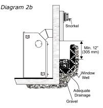
6) The arrow on the vent cap should be pointing up. Insure that the 1-1/2" clearances to combustible materials are maintained (Dia. 3). Install the termination cap. AstroCap™ or Dura-Vent Horizontal Termination Cap may be used.
