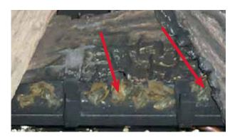
Separate platinum embers and place them on the front of the burner on and around the rock wool. Separate embaglow embers and place over rock wool and platinum embers
