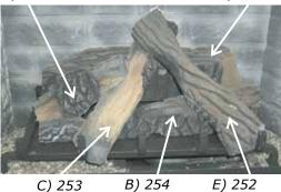
4) Place Log <u>254</u> on the front right side of the burner. Push the back of the log against the 2 brackets with the notch on the bottom right side of the log fitting into the right side of the grate
