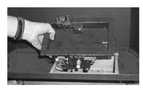
Diagram 3: Lift out Valve Tray Assembly
