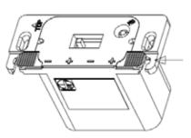
STEP 4 Reinstall wall cover plate with 2 Phillips head screws.
