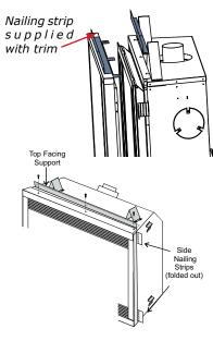
If finishing flush with the Vignette Finishing Trim - bend nailing strips around side trim pieces as shown below.
