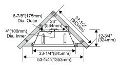
**NOTE:** If this is an outside corner, the minimum distance between the vent and the outside corner is 6" (15cm) with AstroCap termination cap or 12" (30cm) with Rigid Vent termination cap. (For Example Dura-Vent).
