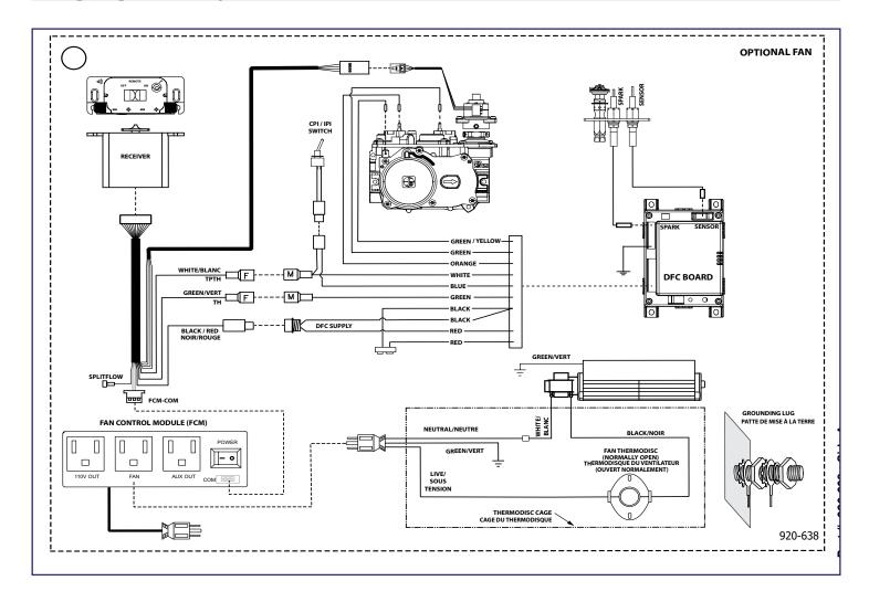
Caution: Ensure that the wires do not touch any hot surfaces and are away from sharp edges. CAUTION: Labelall wires prior to disconnection when servicing controls. Wiring errors can cause improper and dangerous operation.
