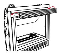
**4.** Install bottom louver assembly by opening bottom louver enough to allow access to attach bottom louver brackets to unit with one screw on each side in locations shown below.
