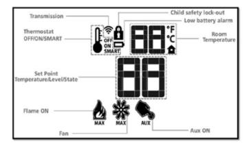
Figure 2: Transmitter LCD Display
