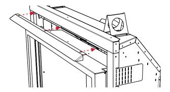
**3.** Install top louver by hooking louver on to brackets installed in Step 1.
