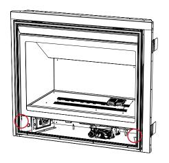
Install safety screen assembly by inserting tabs on assembly into slots on installed Vignette frame (see below). Screen assembly is secured at bottom with magnets.
