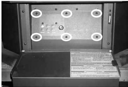
6. Disconnect the manual switch cable and reset cables.
