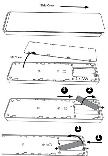
Ensure that the handset batteries are new and inserted correctly.
