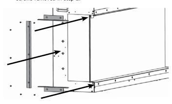
Ensure that the trims are all flush to each other at all 4 corners prior to tightening all 7 screws.
