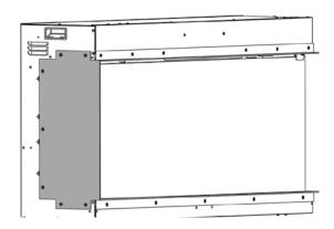
Remove 7 Phillips heads screws and recycle metal side cover. Do not discard screws.
