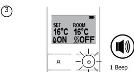
Within 10 seconds, press the button on remote. The coding is finished when 1 long beep sounds from the unit.
