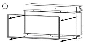
The decorative finishing trim (shown above) would only be installed if this was installed as a single sided. If installed as a two sided/ three side the decorative finishing trim will need to be recycled as it cannot be used.
