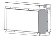
Remove the decorative trim support bracket and recycle (depending on model there may be 2 trim support brackets) Reinstall screws.
