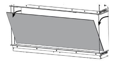
Remove and wash the fuel effect to remove any dust particles. Alternatively clean with a lint free duster.
