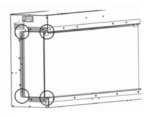
Remove the decorative trim support bracket and recycle (depending on model there may be 2 trim support brackets) Reinstall screws.
