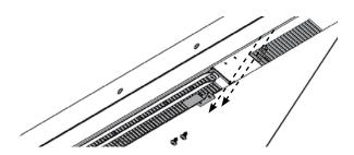
Remove 7 Phillips heads screws and recycle metal side cover. Do not discard screws.
