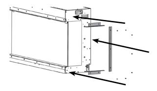
Ensure that the trims are all flush to each other prior to tightening all 7 screws.
