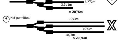
**Example** 2 x 923-835 Mood Lighting strip kit & 1 x splitter and 1 x wiring from appliance to LED mood lighting used. See below.
