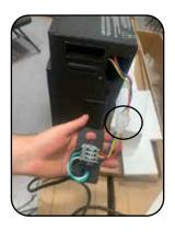
Install the wire harness & cover plate and 120 VAC power cord to the appliance and secure with the 2 x Philip head screws removed in step 2.
