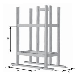
NOTE: The appliance must be installed on a flat, solid, continuous surface (e.g. wood, metal, concrete). which must be the full width and depth of appliance. This may be the floor, or raised up on a platform to enhance its visual impact.
