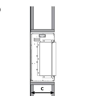
**NOTE:** The appliance must be installed on a flat, solid, continuous surface (e.g. wood, metal, concrete).which must be the full width and depth of appliance. This may be the floor, or raised up on a platform to enhance its visual impact.
