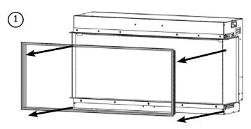
The decorative finishing trim (shown above) would only be installed if this was installed as a single sided. If installed as a two sided/ three side the decorative finishing trim will need to be recycled as it cannot be used.
