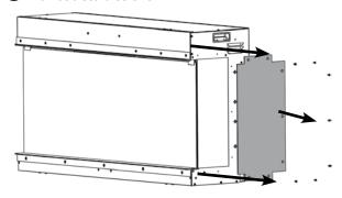
Secure the top/bottom trim using the sames screws removed in step 2. Do not tighten. Secure back trim using same screws removed in step 2.
