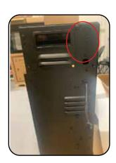
Remove the wire harness & cover plate from the appliance by removing the two Philip head screws from the side of the appliance as shown below. Disconnect the Molex connector and remove the wire harness & cover plate. Once removed recycle or keep the wire harness & cover plate for future use.
