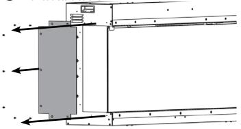
Secure the top/bottom trim using the sames screws removed in step 2. Do not tighten. Secure back trim using same screws removed in step 2.
