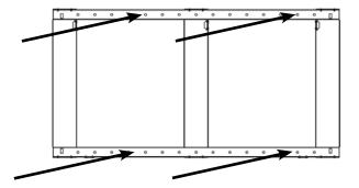
2 Hook appliance onto the wall mounting bracket as shown above.
