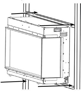
3 Secure appliance to framing as shown below with supplied black wood screws.
