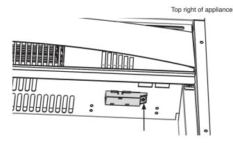
Slide the RF Receiver right and lower out of its location.
