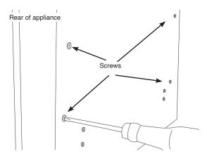
Remove the 2 side covers by carefully sliding forward.
