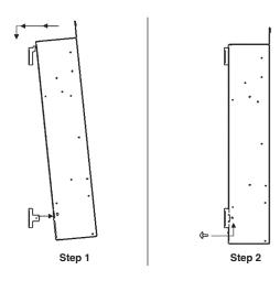
Use two No. 6 x 12 screws from the kit to fix the fire through both sides into the holes in the lower bar.
