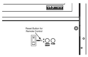
Resetting of the remote control is necessary if the appliance operates wrongly due to external interference signal and the remote control is not in use.
