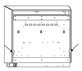
$\boldsymbol{-}$  Let the legs spring back once over the top bar to engaged with the lower bar.
