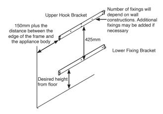
Use a spirit level to check the bars are straight. Mark the positions for the retaining screws. Remove the bracket and drill the holes.
