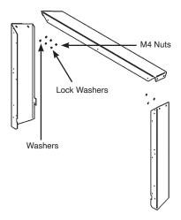
Insert threaded studs in the sides through the holes in the end flanges of the top.
