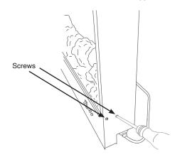
Remove the 4 screws on the back (2 on either side of the back).
