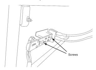
Replace in reverse order ensuring the wires and connectors are put back in exactly the same configuration.
