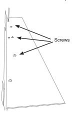
Remove the 3 screws at the top of the back of the appliance. SUPPORT THE HEATER ASSEMBLY WHILST REMOVING THE SCREWS.
