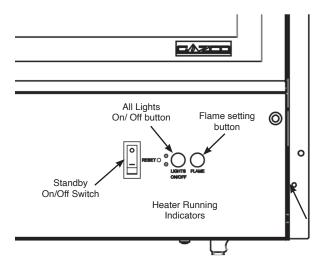
Note: The appliance will lose the memory for the light functions when the switch is set to the Off Position or the remote runs out of power.
