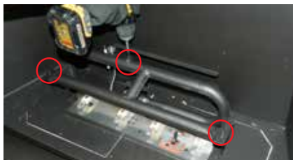
Diagram 2: Slide burner assembly to the right—then remove.
