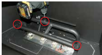
Diagram 2: Slide burner assembly to the right—then remove.
