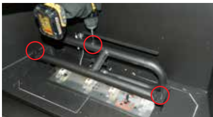
Diagram 2: Slide burner assembly to the right—then remove.
