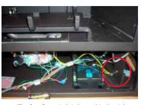
The Surefire switch is located in the right corner of the bottom louver/panel.
