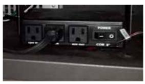
8) Plug fan power cord into the Fan Control Module (FCM) then plug in the FCM. The switch is on when pushed to the left. (Shown in OFF position above)
