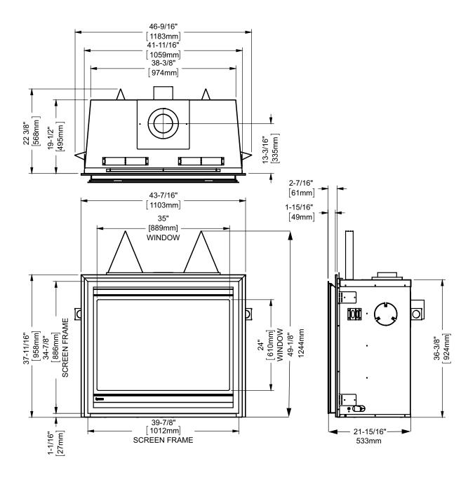
Note: Gas connection is from the right hand side of the appliance & electrical connection on left hand side of the appliance. A metal receptacle box is supplied/installed with the appliance to make all 120 volt electrical connections.
