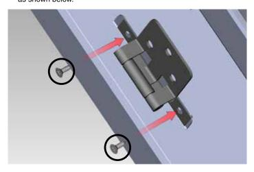
3. Flip the hinges down to  $90^{\circ}$  - line up the lower premium front as shown below.
