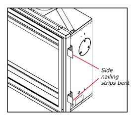
Side nailing strips can be adjusted from 1/2" to 2-5/8".
