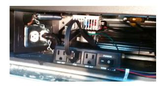
11. Plug in the fan power cord to the Fan Control Module into the outlet marked "Fan". Plug the FCM-COM wire from the remote control wiring harness into the location on the Fan Control Module marked "COM". Turn the switch on the Fan Control Module to the ON position. ON is to the left. The "O" is the off position
