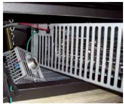
5) Lift the fan housing upwards and slip it over the two mounting studs. (use of dish soap will help the rubber grommets slide down over the pins)
