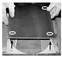
**Before proceeding to Step 8**, inspect condition of all gaskets. DO NOT install parts with damaged gaskets. Replace if necessary with spare gaskets supplied.
