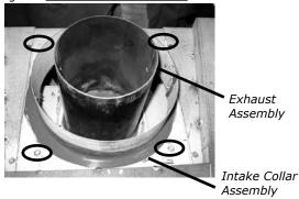
12. From the outside rear of the firebox: install the intake cover plate with 4 - 1/4" x 1/2" screws. Ensure all screws are tight, but do not over tighten. All 4 screws must be used.
