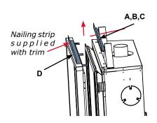
Determine the total thickness of facing material (e.g. drywall or wood plus ceramic tiles) to allow the finished surface to be flush with the front of the unit. Total facing thickness can vary from 1/2" (13mm) to 3-1/8" thick.
