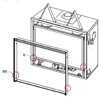
**6**. Line up the tabs on the screen assembly with the slots in the outer frame and lower gently into place. Bring bottom of the screen assembly toward the front of the appliance until it comes into contact with the magnets
