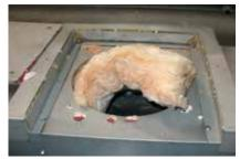
From the outside back of the firebox: locate the insulation deflector and bend completely upwards flat against the back of firebox.
