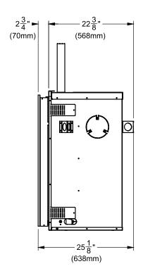
Note: Gas connection is from the right hand side of the appliance & electrical connection on left hand side of the appliance. A metal receptacle box is supplied/installed with the appliance to make all 120 volt electrical connections.
