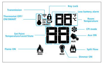
Figure 2: Transmitter LCD Display
