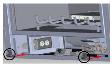
2. Attach the each hinge to the corresponding bracket with 2 screws as shown below.
