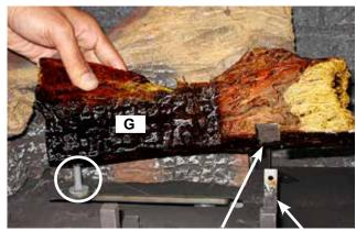
Notch - Log G Burner Grate Tab
