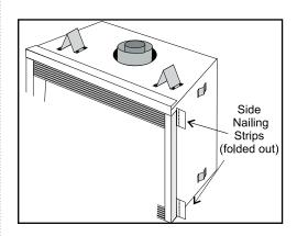
If finishing flush with the Vignette Finishing Trim-bend nailing strips around side trim pieces as shown below.
