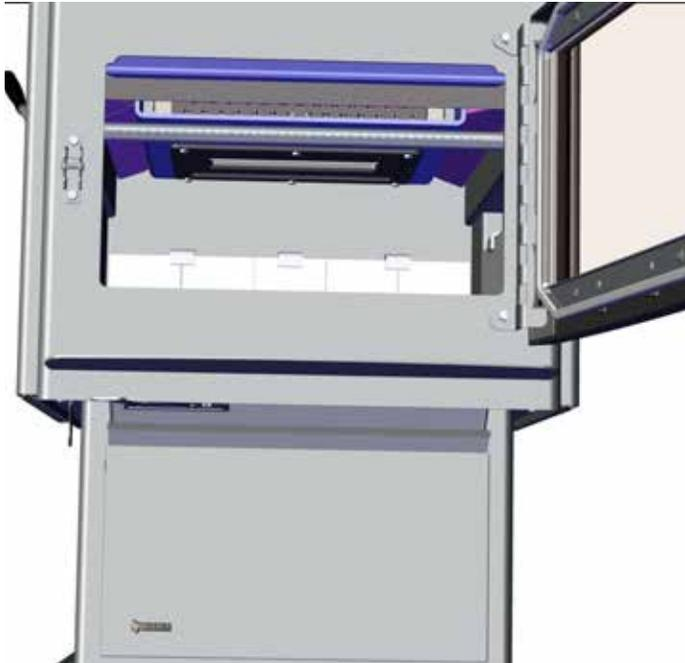
3. Loosen the 3 rear nuts, then remove 3 front nuts. Support the Bypass Door from the front /back and slide forward to remove Bypass Door Assembly.
