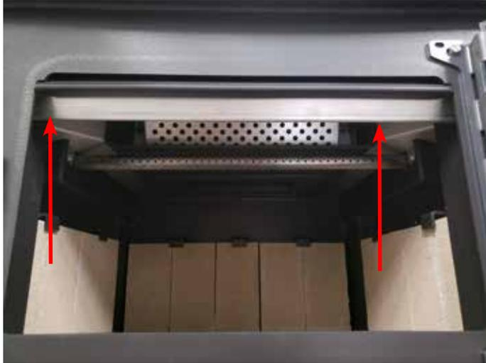
3. **Correct Install:** Ensure return edge of smoke deflector is seated within the backside of the glass wash.
