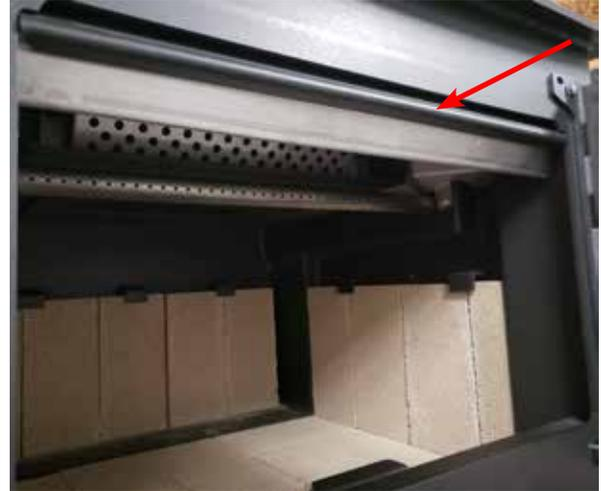
2. To replace the deflector, loosen off both 7/16" bolts and slide deflector upward and out. Install new deflector and hand tighten 7/16" hex head bolts. Ensure positive location of the deflector prior to hand tightening. **WARNING:** Operation of the unit without proper installation of smoke deflector will void warranty.
