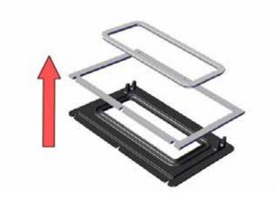
6. Reverse steps to reinstall - ensure the pass rod is seated with the channel on the pass door. (Unit viewed as transparent to facilitate view)
