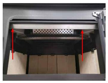
2. To replace the deflector, loosen off both 7/16" bolts and slide deflector upward and out. Install new deflector and hand tighten 7/16" hex head bolts. Ensure positive location of the deflector prior to hand tightening. WARNING: Operation of the unit without proper installation of smoke deflector will void warranty.
