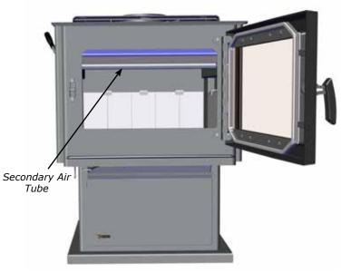
**3.** Grasp secondary air tube firmly with vise grips, using a hammer tap vise grips from right to left until air tube is released from grip. Remove.
