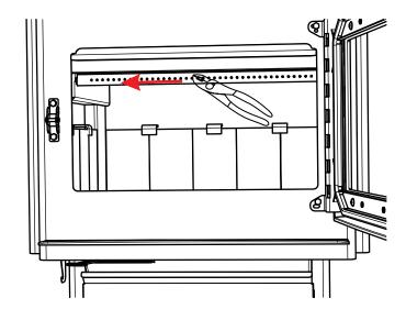
4. To reinstall or replace, first slide left side of tube into hole on left side air channel. Align tab on right side air channel with notch on right hand end of air tube. Firmly grip center of air tube with vise grips, use hammer to tap vise grips from left to right until the tube bottoms out into the air channel on right.
