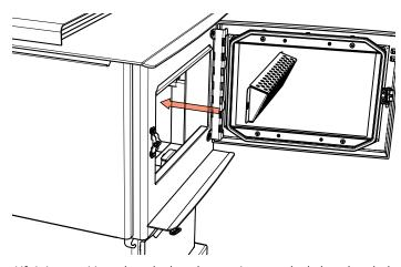
Lift it into position, place the key slot opening over the bolt and push the flame shield down to seat. Tighten the bolt till its SNUG only, do not over tighten. The flame shield should rest at an angle (about 45 degrees) with the thin end at the bottom and the thick end near the top of the stove.
