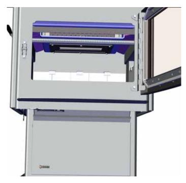
3. Loosen the 3 rear nuts, then remove 3 front nuts. Support the Bypass Door from the front /back and slide forward to remove Bypass Door Assembly.
