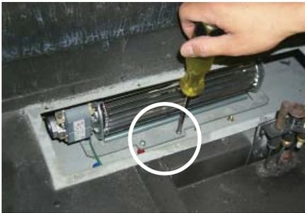
12) Pull Fan Assembly forward, to disengage the fan clip on the rear wall. Then lift the Fan Assembly up and pull through firebox opening.
