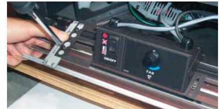
Secure left side with 2 screws.
