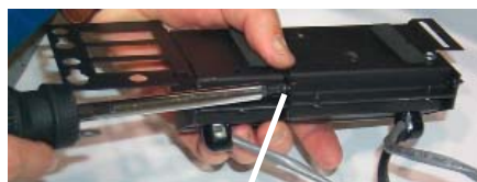
Secure the 2 boxes together with one screw.
