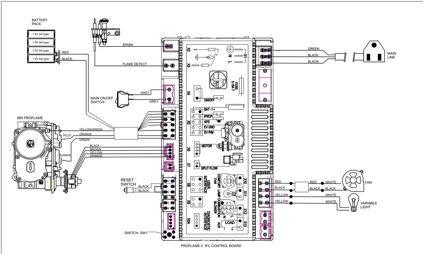
WIRING DIAGRAM WITH OPTIONAL THERMOSTAT
