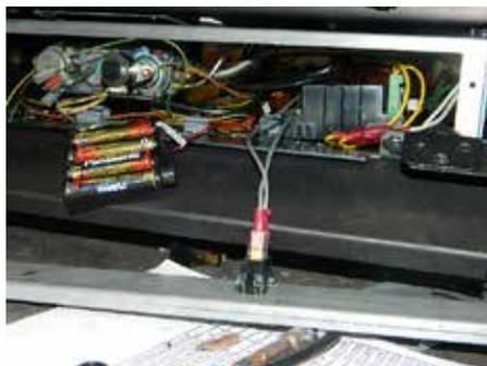
4. Install 4 AA batteries into the box and slide it back to its original place.
