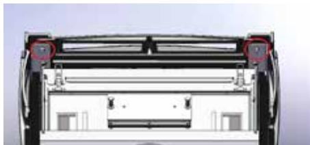
3) Remove light assembly and carefully set aside.
