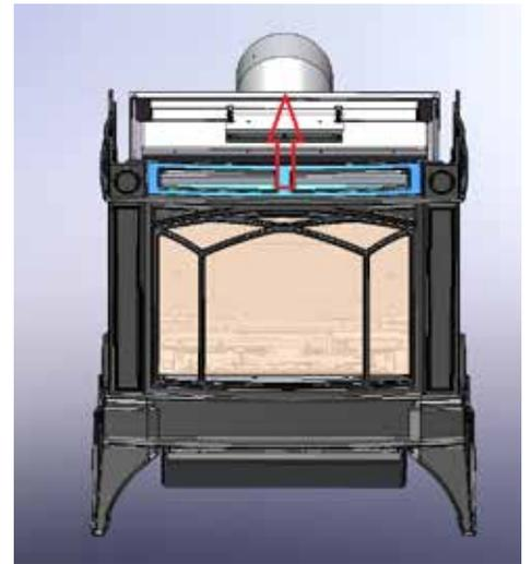
6. Slide safety screen upwards to remove.
