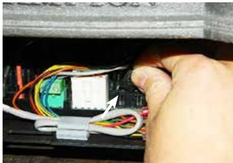
11. Remove NG stepper motor by removing 2 screws in locations shown below. Replace with LP stepper motor, secure in place with 2 screws.
