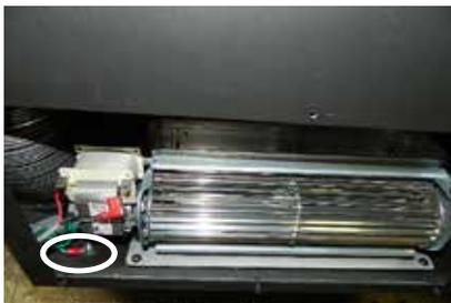
5. Open the bottom cover of the unit by loosening the 2 screws and removing one from the left side of the unit (when facing back of the unit).
