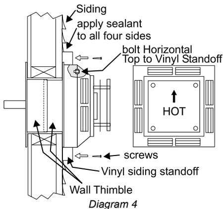
tive wall thimble cover over the vent pipe, then slide the Wall Thimble over the vent pipe.
