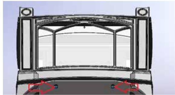
7) Slide the casting out of the base plate and the side bracket key hole slots and lift the front casting off the unit.
