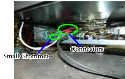
8. Attach the connectors (black and red) of Fan Grey wire to the IFC connectors (black and red). **NOTE: Do remember to follow the wire color code, i.e., black to black and red to red). Refer to the picture above.**
