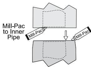
**NOTE: For best results and optimum performance with each approved venting system, it is highly recommended to apply "Mill-Pac" sealant (supplied) to every inner pipe connection. Failure to do so may result in drafting or performance issues not covered under warranty.**
