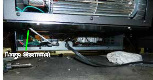
7. Run the fan grey wire through the small grommet power cord from the valve cover plate to the base panel through the large grommet.
