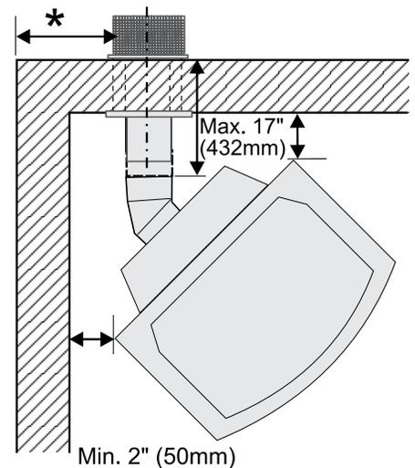
\*If this is an outside corner, the minimum distance between the vent and the outside corner is 6" (15cm). See "F" on the diagram in the "Exterior Vent Terminal Locations" section.
