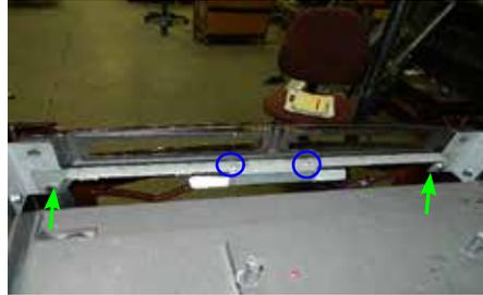
*Lift light assy bracket off bolts to install bulb
