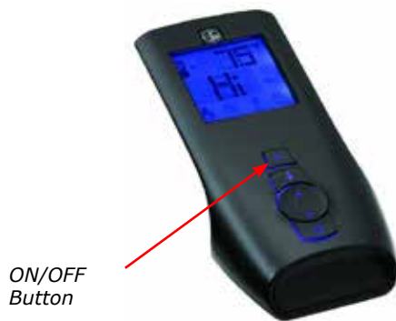
Diagram 2 Remote shown in Manual Mode on Hi
