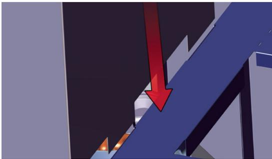
*Diagram 2 - Lower tabs on panel aligned with base*
