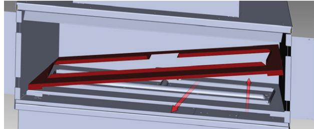
HZO42 only- remove 6 screws in locations shown below to access DC supply.
