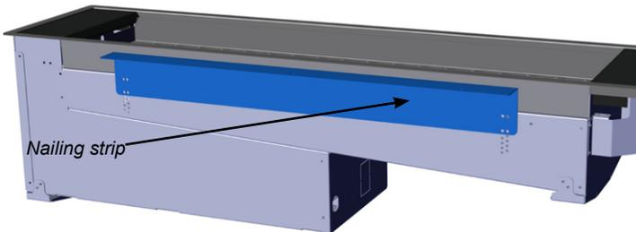
Side nailing strips are adjustable in 1/4" or 1/8" increments. Each hole on the inside line is 1/8", each hole on the outside line is 1/4". Determine the thickness of the finishing material before adjusting the nailing strips.
