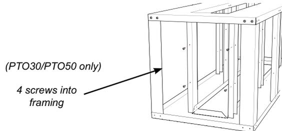
In the diagram below the outer box is installed. To install the outer box, line up the keyholes on the box with corresponding screws (installed in previous step) on the framing kit. When the box is in position, tighten the screws. (PTO30/PTO50 only)
