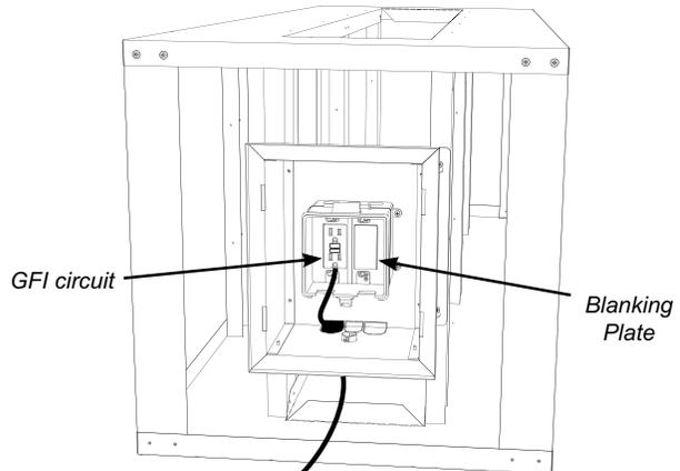
5. Plug in the supplied AC adaptor and run the wire through the bottom of the outer box, be sure to use a grommet to protect the wire.
