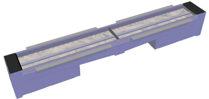
6. Install units together into framing (refer to framing section). Secure in place with nailing strips.
