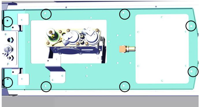
11. Lift valve assembly up and out.
