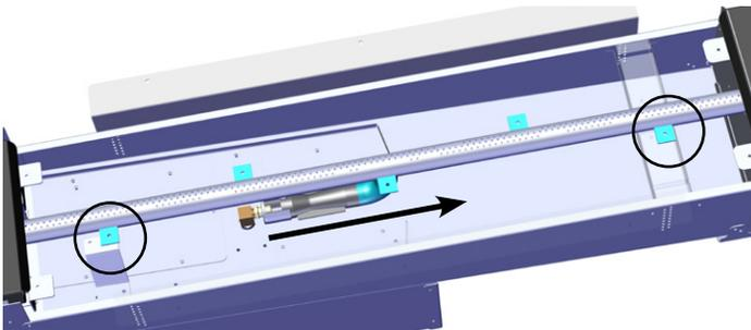
6. Remove 6 screws on valve access cover.
