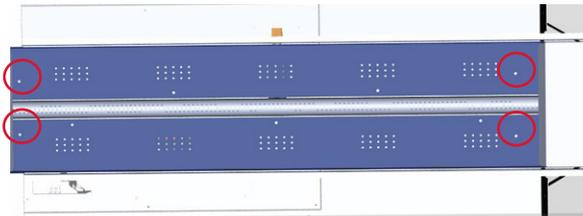
4. Slide burner away from burner orifice and lift up to remove burner assembly.
