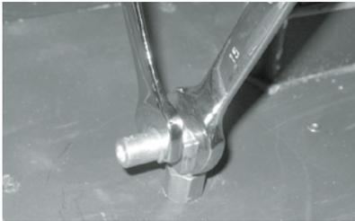
8. Pull off the pilot cap to expose the pilot orifice. Using a 5/32" allen key, remove pilot orifice and replace with LP pilot orifice.
