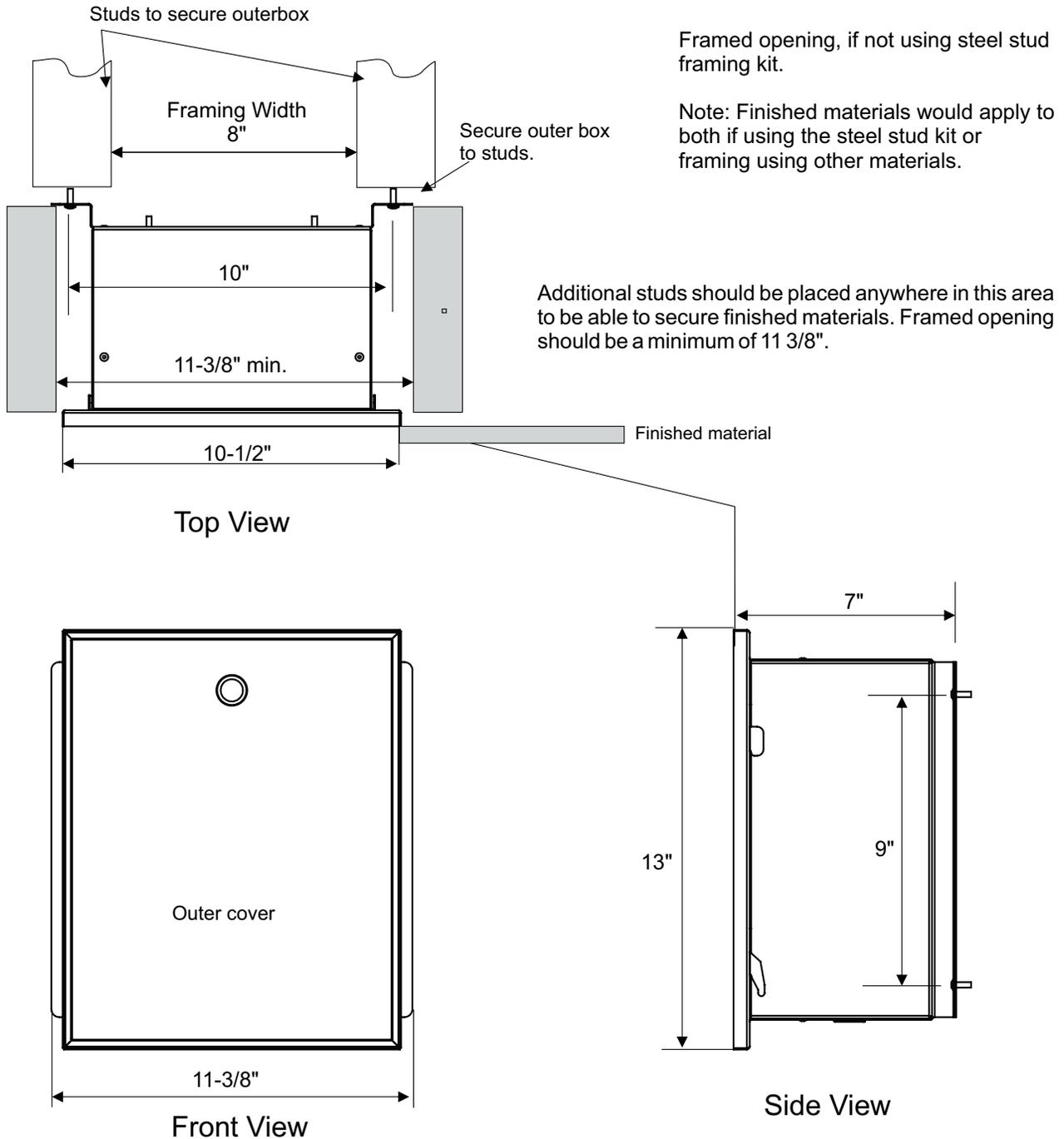
The front outer cover may also be covered with finishing materials if desired. Ensure that the outer cover when using finished materials, that it may be removed if access is ever required to the GFI circuit.
