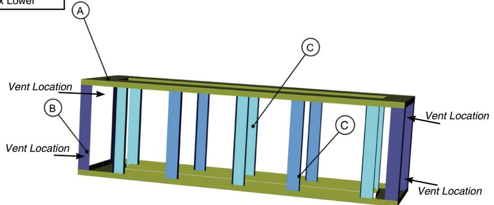
**Important Note:** Four (4) ventilation grills are required for all the PTO60 steel stud framing kit. This is to alleviate moisture and allow for air to circulate underneath this burner. Minimum required size: 20" sq (508 mm<sup>2</sup>) ea.
