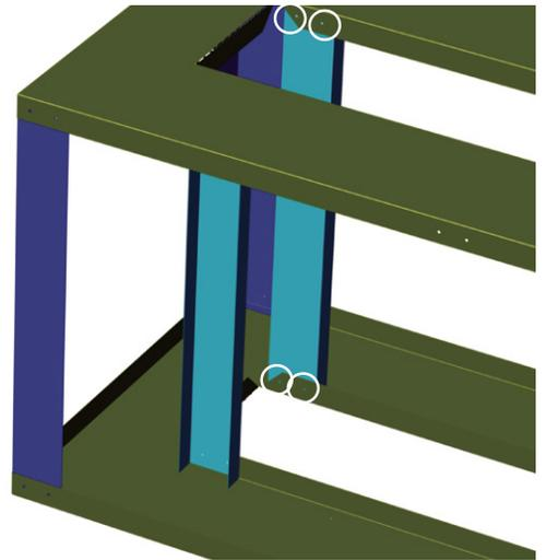
Diagram 5 - Inside vertical support screw locations
