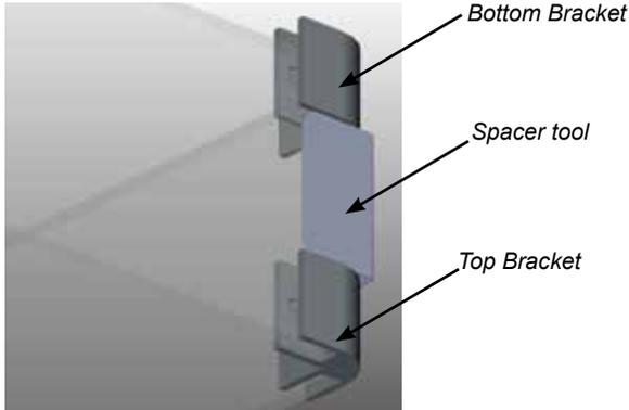
5. Secure bottom corner brackets with nylon fasteners in each corner.
