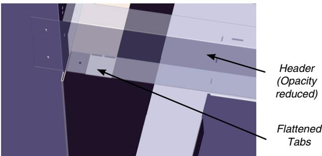
*Diagram 3 - Bend tabs flat, panels is supported on headers.*
