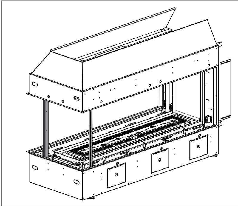
NOTE: UNDER NO CIRCUMSTANCE MAY THE END FIREBOX GLASS BE REMOVED FROM THE FIREPLACE. ONLY REMOVE THIS GLASS PANEL WHEN TRANSPORTATION SUPPORT BRACKETS ARE IN PLACE.
