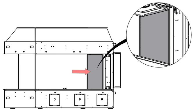
5. Clean panels with a cloth. Add the desired media or logs before installing the inner firebox glass. See this manual for instructions on how to install the firebox glass.
