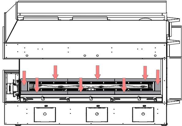
5. Slide the side glass panel #4 into the bottom side bracket and secure the side glass by mounting the top bracket and tightening the 2 screws.
