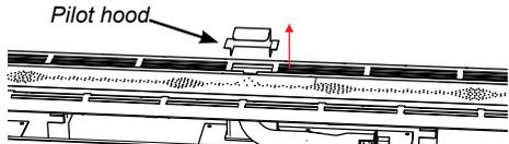
11. Remove the trim cover on right side of burner by lifting off. Also remove the burner surround by sliding to the left and lifting off. Also remove the perforated air diffuser on the right side of the burner.
