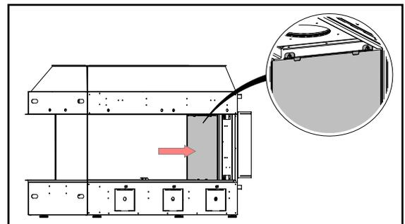
6. Clean panels with a cloth. Add desired media or logs before installing the inner firebox glass. See this manual for instructions on how to install firebox glass.
