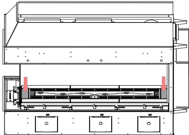
4. Install the 2 screws loosely on the sides of the firebox and place the #3 side panel in the sides of the firebox as shown below.
