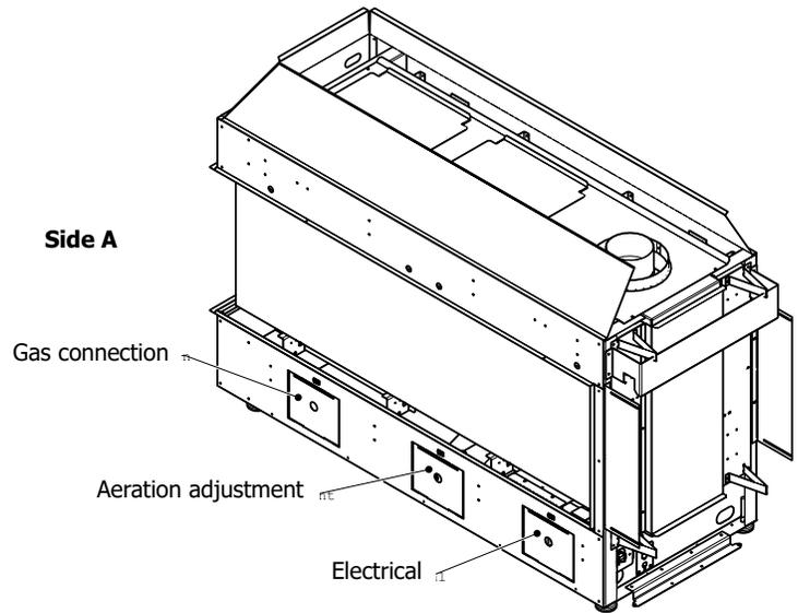
1. Identify the access panel and remove the corresponding outer trim panel by lifting it up and off (centre panel shown opposite).
