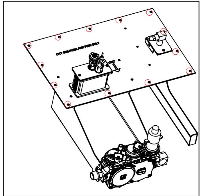
10. Lift valve tray out partially and disconnect flexible gas connection on the valve inlet side. Remove the valve tray and replace it with the new valve tray & valve assembly gasket.
