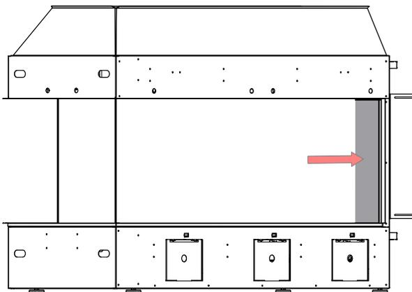
9. Clean the outer panels with a cloth before installing the safety outer barrier glass. To install the safety glass, see this manual for instructions.
