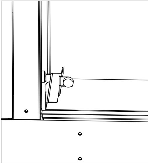
9. Slide the side outer #6 glass panels between the wall and the barrier stopper bracket. If the unit does not have a barrier stopper, stick the side outer panels to the magnets.
