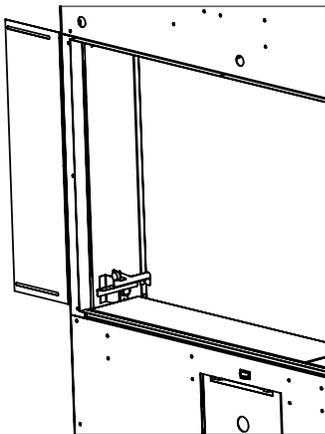
8. Slide the side #5 outer panels between the wall and the barrier stopper bracket. Repeat steps to install the remaining three #5 outer panels using a barrier stop where required.
