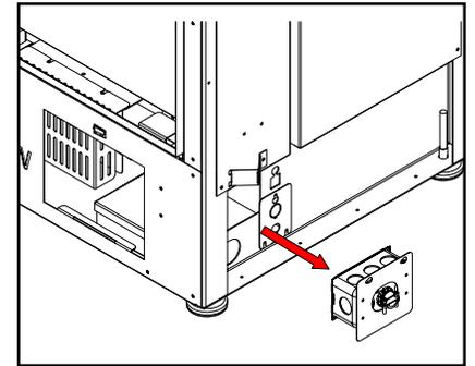
3. Slide electrical box plate towards the back of the unit and then out.
