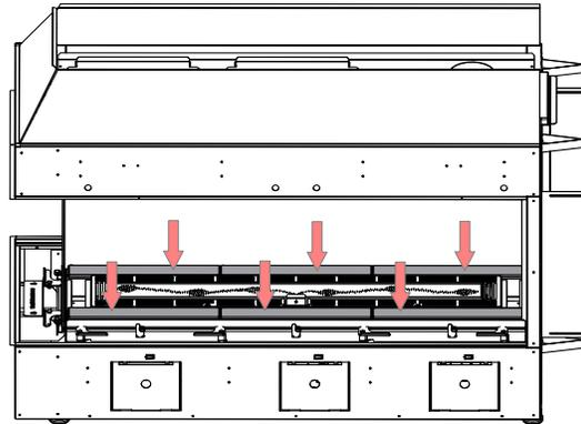
3. Drop the two #2 panels into the firebox on the left and right ends as shown below.
