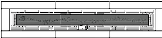
2. Install the 3.5 lb box of black charcoal glass and 1 lb of Andiron embers around the burner. Make sure the burner surround is only 50% covered.
