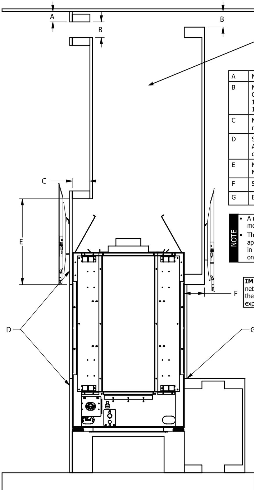
**Important:** The chase enclosure must be fully open the full width, height and depth above the fireplace as per the requirements noted in the framing section for both bench/flush installations.
