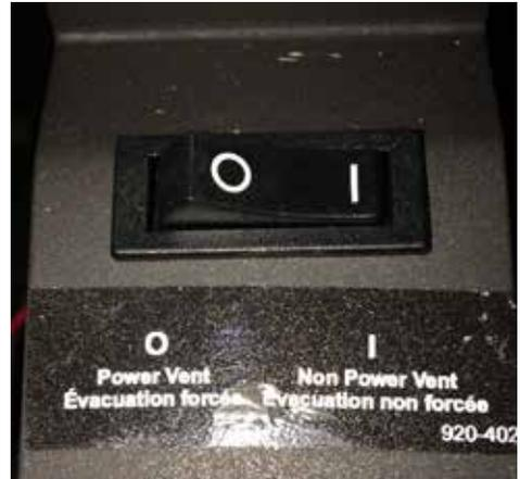
**NOTE** This switch would have been positioned at time of install and should never have to be moved from one position to another. This switch is hidden to avoid the home owner having the switch in wrong position.
