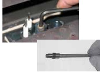
16. Reinstall pilot cap and pilot retainer clip.
