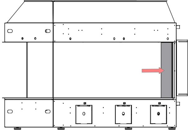
10. Clean the outer panels with a cloth before installing the safety outer barrier glass. To install the safety glass, see this manual for instructions.
