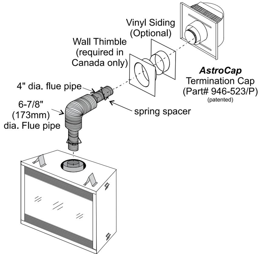
**If longer runs are needed, the Regency Direct Vent system (Flex) # 946-516 includes all the parts needed to install the P36E with a maximum 10' run.**
