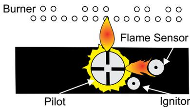
Incorrect flame pattern will have small, probably yellow flames, not coming into proper contact with the rear burner or flame sensor.
