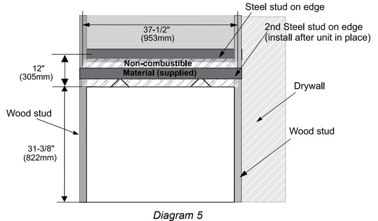
**NOTE:** If using flush louvers and safety screen the steel studs and non-combustible material are not required. Wood studs and drywall may be used. See framing and finishing for details.
