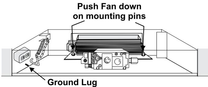
4. Connect the power cord and fan ground wires to the ground lug. Refer to wiring diagram.
