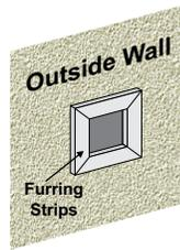
**Note:** If installing termination on a siding covered wall, furring strips must be used to ensure that the termination is not recessed into the siding.
