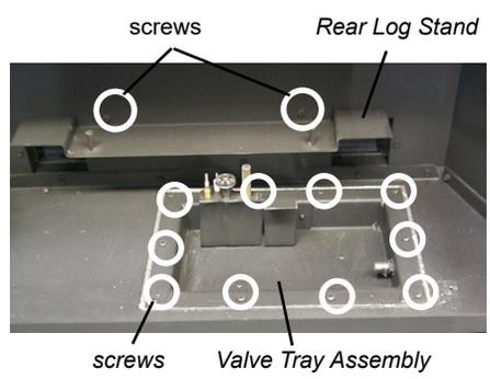
Diagram 2: Rear Log Stand and Valve Tray Assembly
