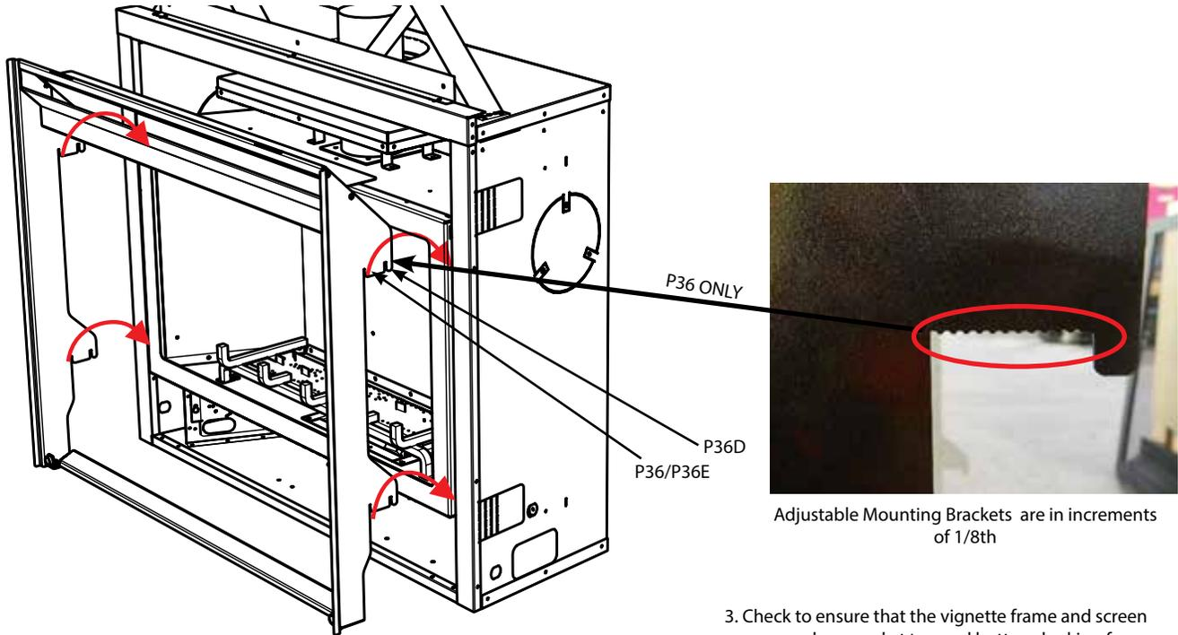
2. Slot the tabs on the inner Vignette frame with safety screen into the corresponding slots in the outer Vignette frame as shown below.
