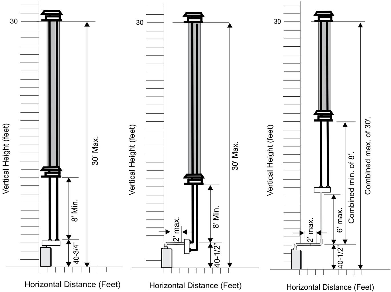
The shaded area in the diagrams show the allowable vertical terminations.
