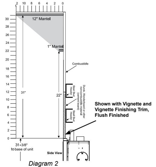
**Note:** Secure the non-combustible board (supplied) directly above the unit as shown. Install a steel stud directly above the unit as shown to secure the non-combustible material.
