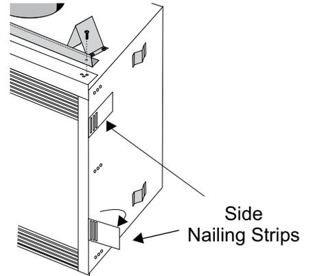
If finishing flush with the Vignette Finishing Trim - bend nailing strips around side trim pieces as shown below.
