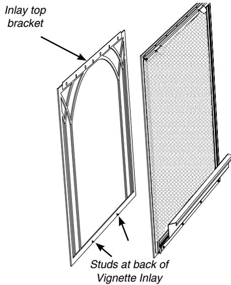
3. Position the Inlay so it is exactly centered from side to side and top to bottom within the Inner Vignette Frame.
