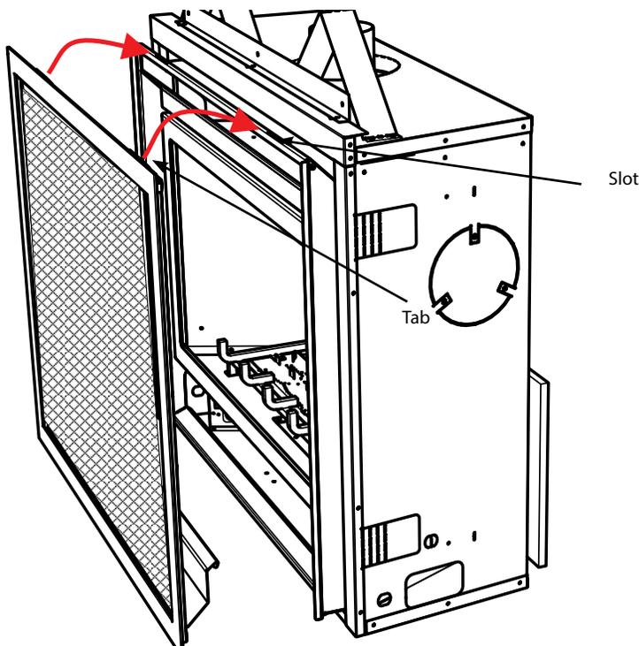
3. Check to ensure that the vignette frame and screen are evenly spaced at top and bottom-looking from side. If it is not evenly spaced, simply lift up the corner and pull gently towards you until adjusted.
