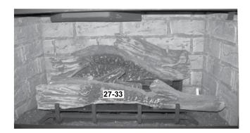
6) Fit the groove in  $\log 27-34$  into the tab on the right side of the burner. Rest the other end of  $\log 27-34$  on the notch in  $\log 27-33$ .
