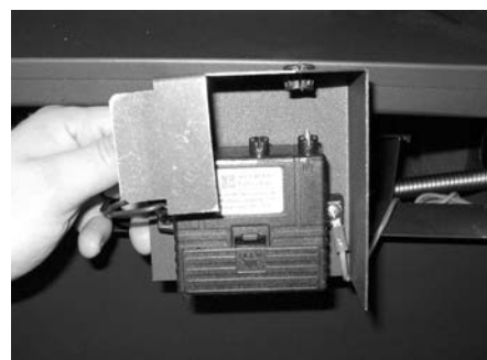
DC Spark Box Bracket Assembly removed from firebox.
