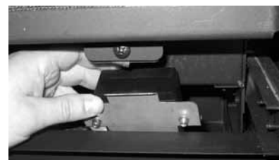
DC Spark Box mounting plate partially removed.
