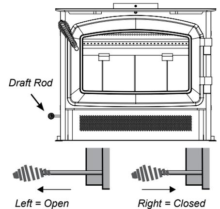
As well as a primary and glass wash air system, the unit has a full secondary draft system that allows air to the induction ports at the top of the firebox, just below the flue baffle.
