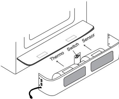
**CAUTION:** Label all wires prior to disconnection when servicing controls. Wiring errors can cause improper and dangerous operation.
