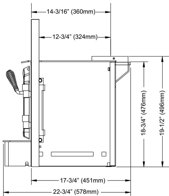
Regency Inserts are designed to use either a 5.5" (140mm) or 6" (152mm) flue.
