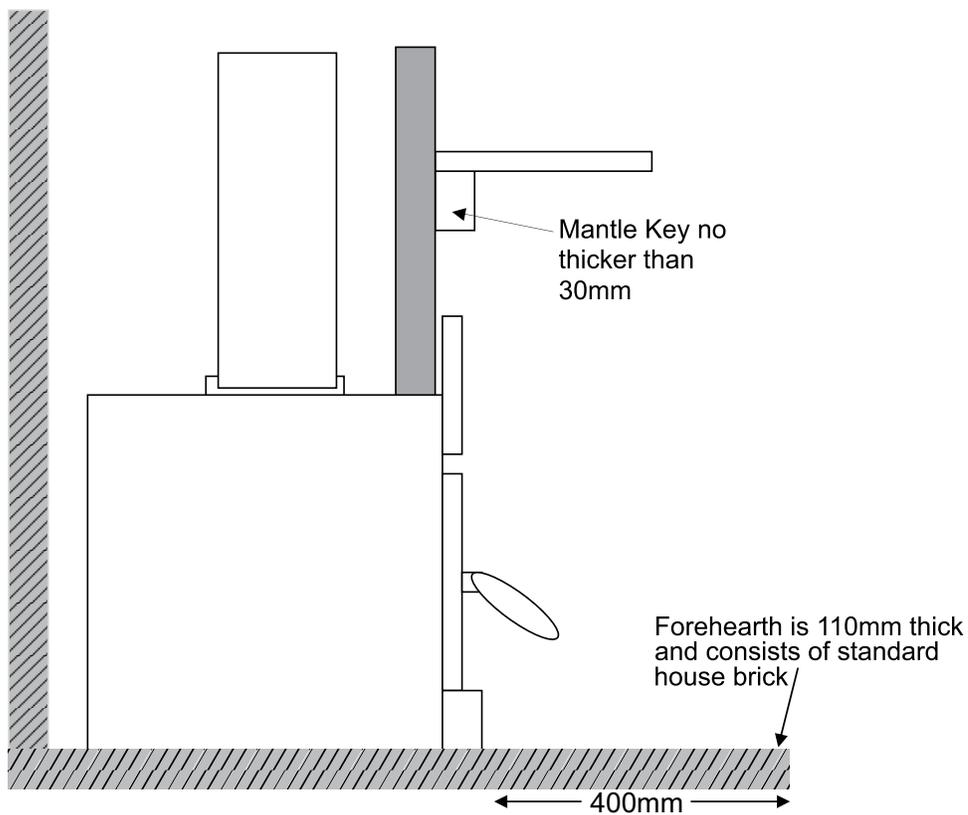
**NOTE** - If using 30mm cement sheet the hearth will need to extend to 820mm
