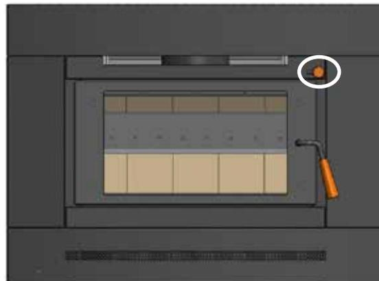
7. Install knob on damper control rod.
