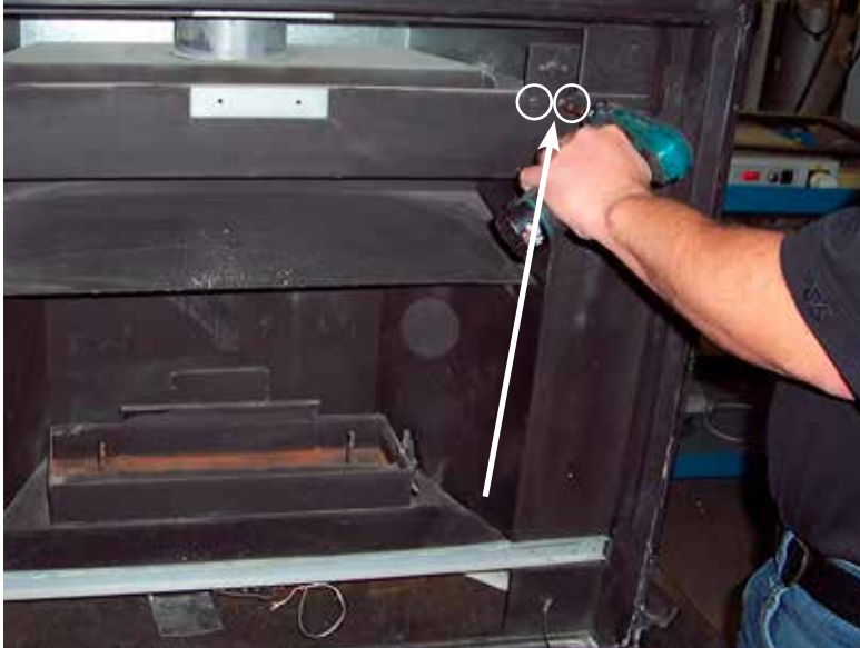
Remove 2 screws - remove Thermodisc Bracket
