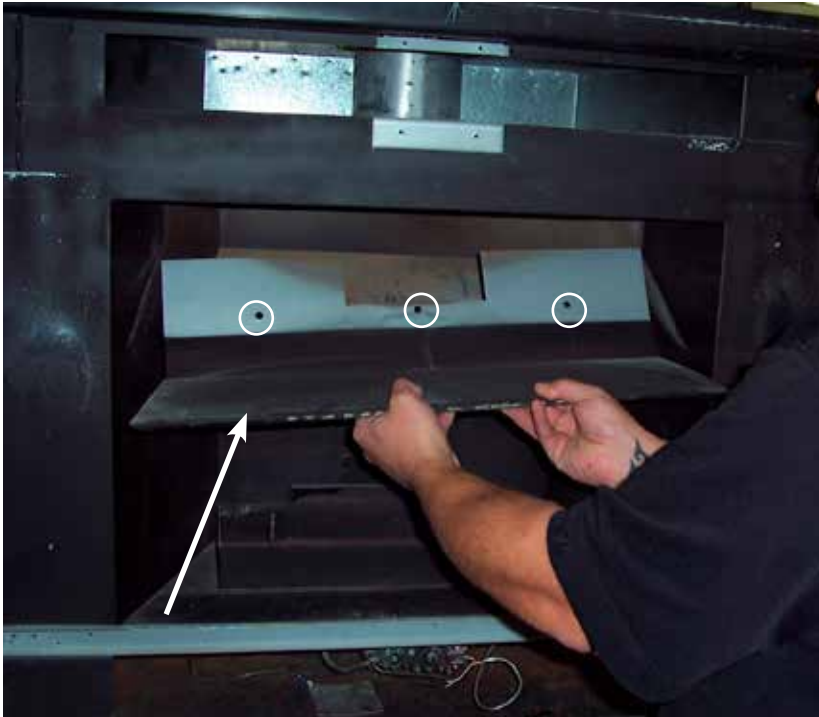
Remove 3 bolts and nuts to remove heat deflector.
