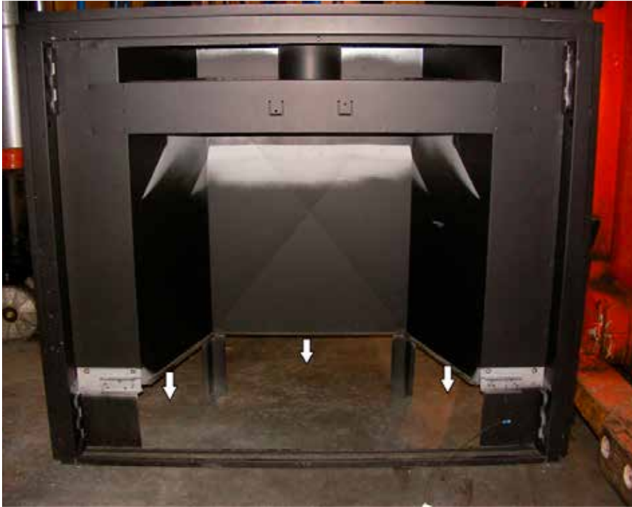
Diagram 6.9 Edges must be flush to allow proper seating of the E18E outerbox.
