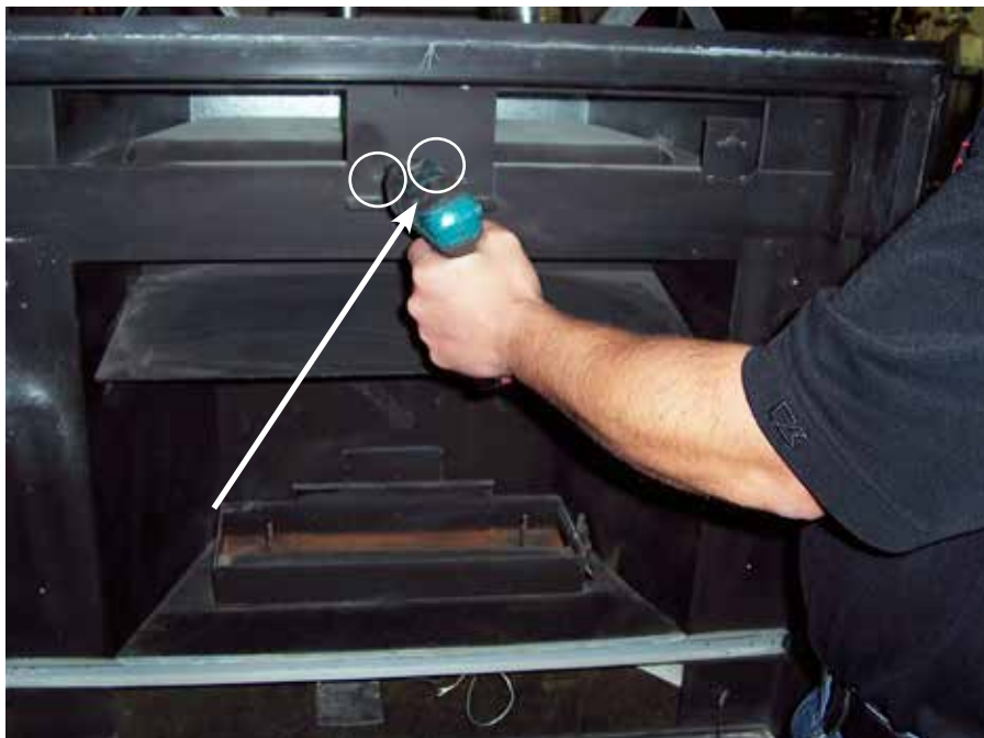
Remove 2 screws - remove Top Bracket
