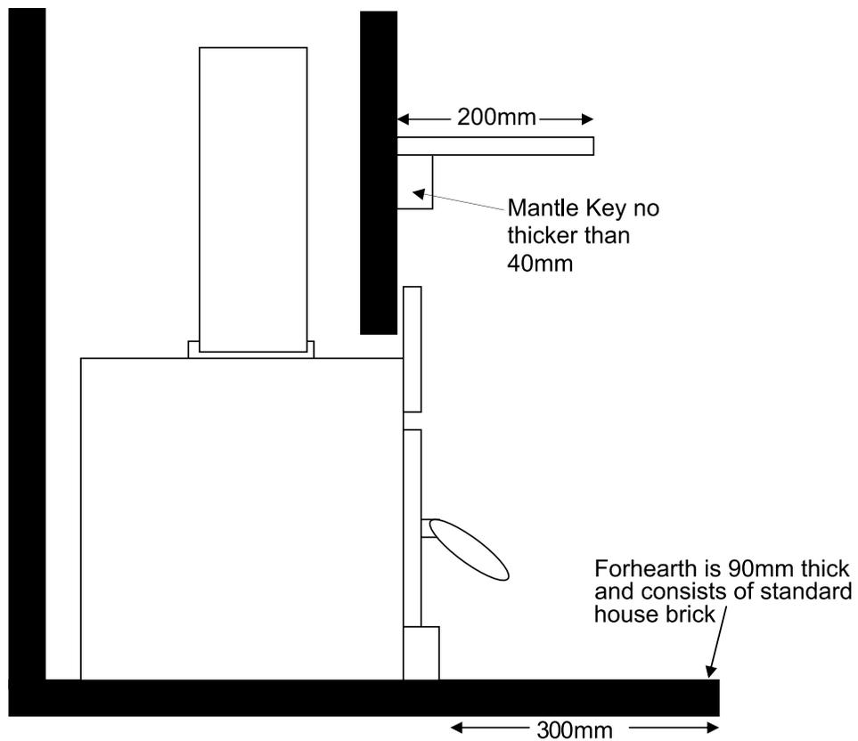
NOTE: If using 6mm cement sheet the hearth will need to be extended to 400mm.
