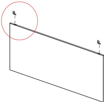
3. Manoeuvre in back panel to the back wall of the unit—secure in place with 2 panel clips and 2 screws.
