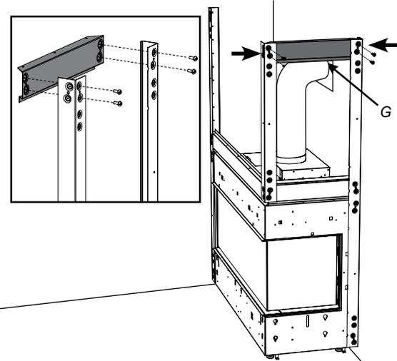
11. Identify H and attach to both front corners C and F with 2 screws on each side.
