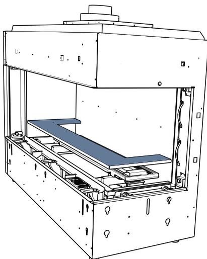
4. Slide the supplied bottom corner bracket behind the small panel (1) and the back and side walls, in the orientation shown below.
