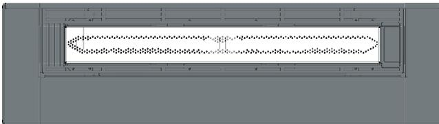
3. Place the various sized fire balls as shown. Ensure the fire balls do not cover any of the burner ports.
