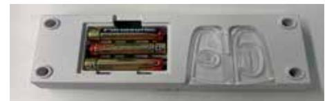
Figure 3: Battery compartment
