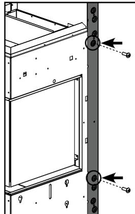
5. Slide unit against wall and line up part C's with studs in the wall. Attach both part C's to studs with at least two screws each; one at the top, and one near the unit (as seen below).
