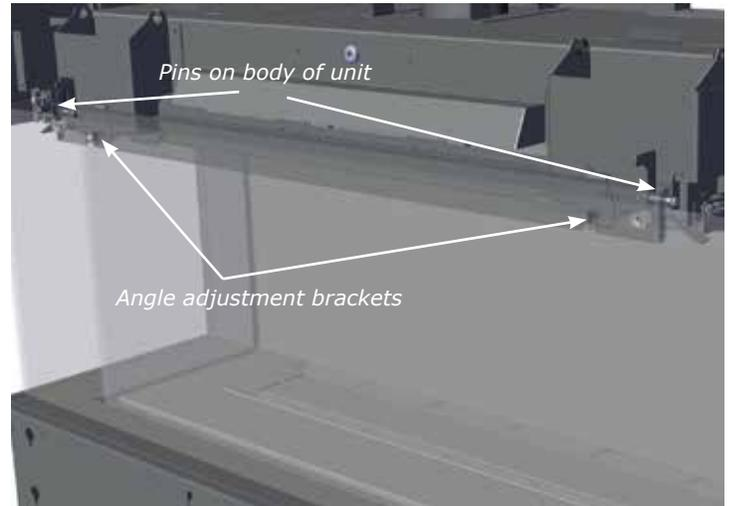
**Note:** If the outer safety glass panels do not sit at 90° and angle too far inward or outward, remove the glass panel and adjust the screw of the panel angle bracket. Turn the panel angle bracket screw in 1/4 increments—reinstall panel to check.
