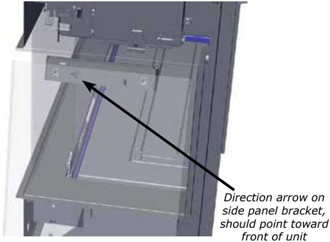
5. Lift up the side panel with the supplied glass clamps (see procedure on previous page). Tilt the side of the glass panel inward and lift up and underneath the upper side panel and hook the 2 outer hooks on to the pins, there is also a panel angle adjustment bracket for the third hook.
