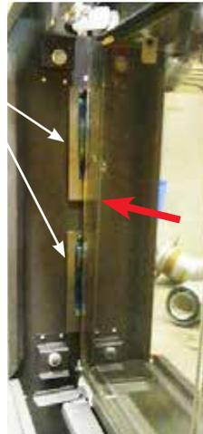
4. With the springs compressed, close the 2 clamps at the bottom and 2 clamps at the top, by turning inward, to secure the glass in position. For the 3 sided unit, repeat on the opposite side.
