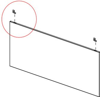
3. Manoeuvre in back panel to the back wall of the unit—secure in place with 2 panel clips and 2 screws.
