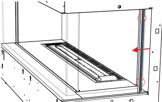
*Loosen 2 screws from inside the firebox to remove the side drywall trim pieces*
