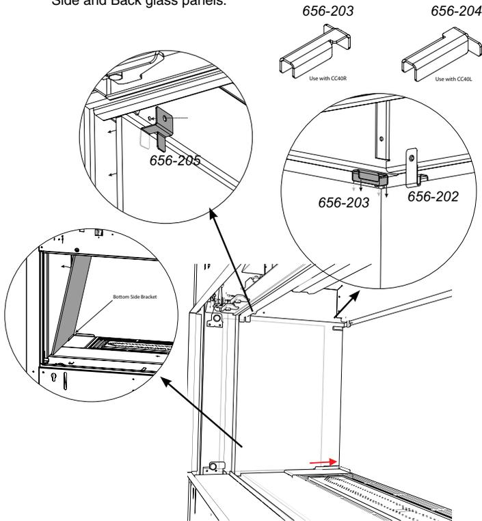
7. Reinstall inner ceramic firebox glass panels (see manual for instructions).
