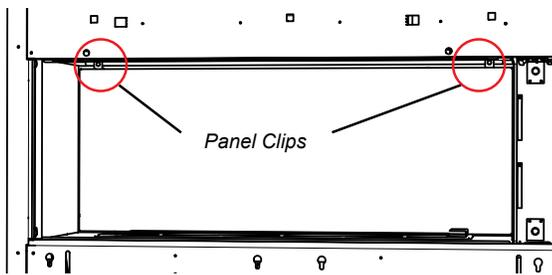
4. Install panel clip into the slots at the top of the side panel as shown.
