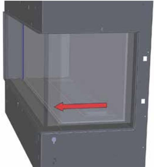
5. Lift up the side panel with the supplied glass clamps (see procedure on previous page). Tilt the side of the glass panel inward and lift up and underneath the upper side panel and hook the 2 outer hooks on to the pins, there is also a panel angle adjustment bracket for the third hook.
