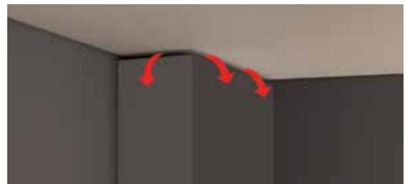
The ventilation opening may be fully open at the top of the enclosure. This type of ventilation opening would be used when the top of the enclosure is not visible from above and where the ceiling within the room is higher than normal. When creating this type of ventilation opening, measures should be in place to avoid having objects of any type falling or be thrown into the ventilation opening. Mesh screen or other preventative measures should be put in place.
