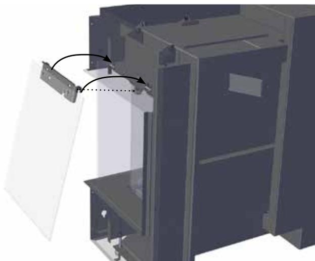
**Note:** If the outer safety glass side panels angle too far inward or outward, remove the side glass panel and adjust on the panel angle bracket, see details on previous page.
