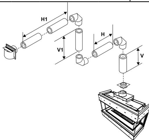
**Vertical Terminations - Rigid Pipe 4" x 6-5/8" (Non Power Vent)**
