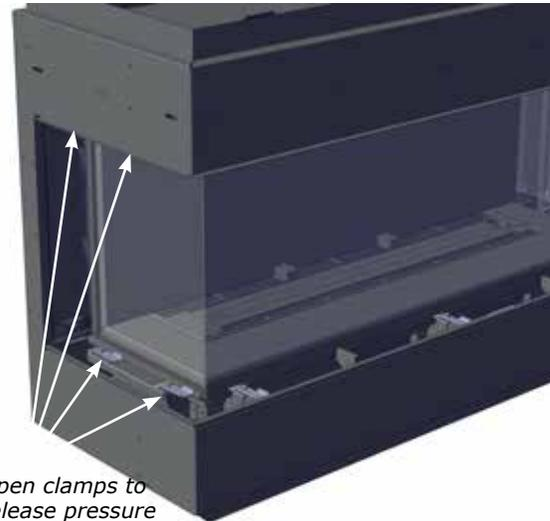
6. Lift up the front panel using the supplied vacuum clamps and position into the lower front channel—ensure the front panel is accurately centered—with the front panel in position—secure in place by closing the 3 lower clamps and 4 upper clamps.
