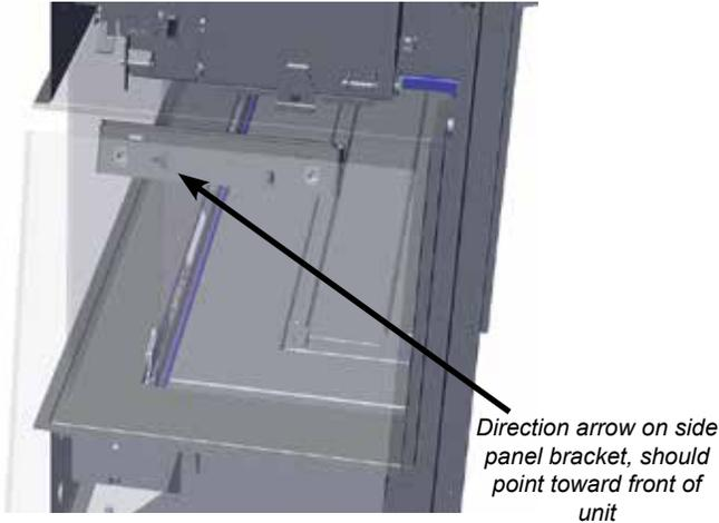
**Note:** The side frame upper panel was made transparent to better illustrate the install (this area is not visible when installing glass).
