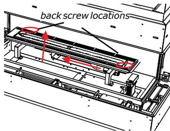
12. Remove burner orifice with a 3/8" wrench. Use another wrench to hold on to the elbow behind the orifice. Discard orifice. Reinstall new burner orifice LPG stamped #53 and tighten.
