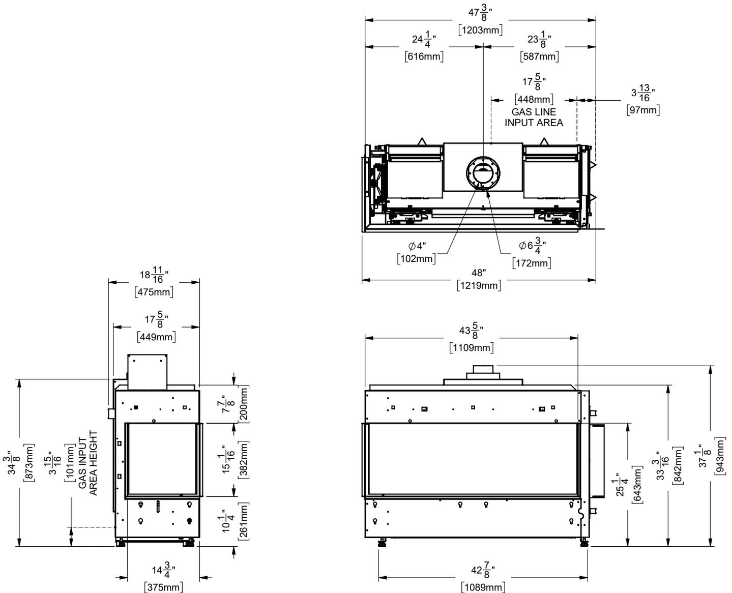
**Note: Electrical connection on left hand side of the appliance.
