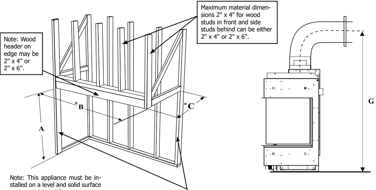
Note: This appliance must be installed on a level and solid surface such as a plywood floor which must be the full width and depth of the appliance.
