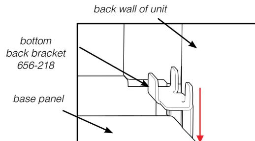
5. Carefully manoeuvre the back glass panel (2) to the back wall of the firebox. Center the glass panel and position bottom of panel into brackets installed in step 4. Place the 2 top back brackets on the top edge of the glass and secure to the unit with one screw on each side once back glass panel is in position.
