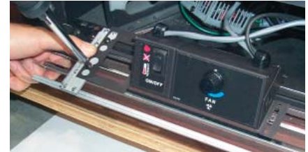
Secure left side with 2 screws.
