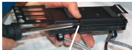
Secure the 2 boxes together with one screw.
