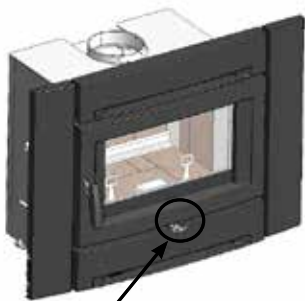
Primary Air Damper Left - Open Right - Closed
