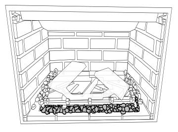
5. Spread the black/white embers along the front panels. When logs 6, 7, and 8 are installed, ensure the embers are not preventing proper log placement. It is also possible to add the embers after all logs are placed.
