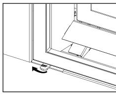
With the pilot on, turn the switch to the right to turn the burner on. Moving the switch to the left will turn the burner off.
