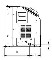
Note: Gas Located on right side of appliance and electrical located on the left hand side of appliance.
