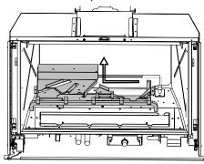
Remove the burner orifice with a 1/2" wrench and replace it with the #38 orifice in the kit. Use another wrench to support behind the elbow when removing/replacing the burner orifice.
