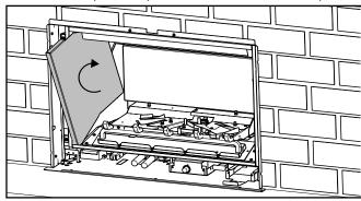
7. Rotate the right panel and push it in until it touches the rear panel.
