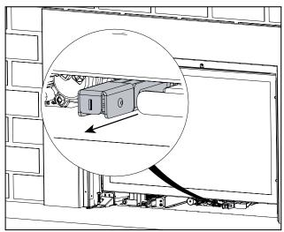
2. Turn gas valve to desired position. If needed, use a flathead screw-driver to turn valve.
