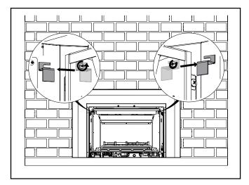
Insert the rear panel and hold in place while installing the left and right panels.
