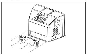
3. Remove the electrical access panel from the left side of the insert by removing five screws.
