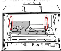
7. Slide the burner tray to the left and out.
