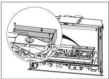
6. Remove the burner tray (2 screws).
