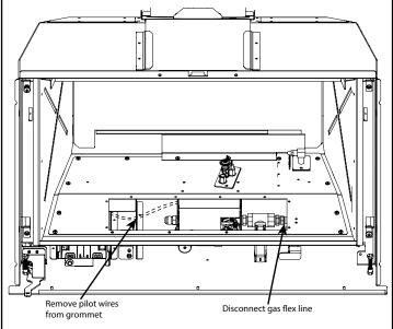
8. Remove the remaining 12 screws and lift the valve tray out.
