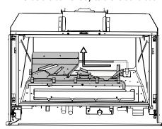
8. Pull off the pilot cap to expose the pilot orifice.
