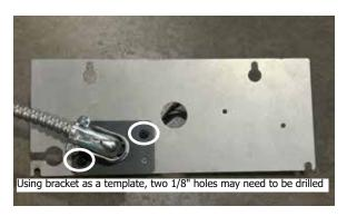
11. Lock the right hand connector using the supplied locking/connector clamp.
