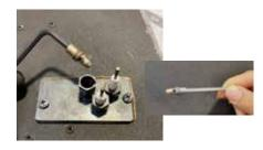
Remove the burner orifice with a 1/2" wrench and replace it with the #52 orifice in the kit. Use another wrench to support behind the elbow when removing/replacing the burner orifice.
