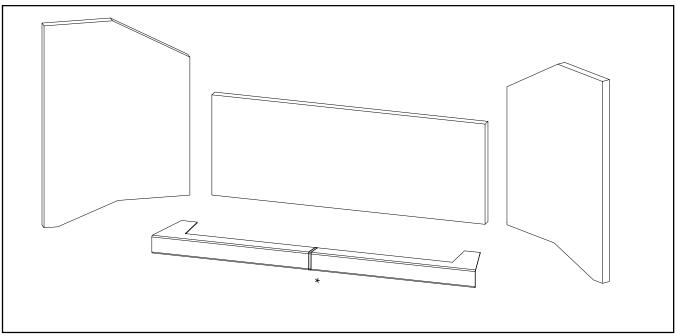
\*The front panel in the steel/black glass panel set is a single part. The front panel in the brick panel set is split into two parts.
