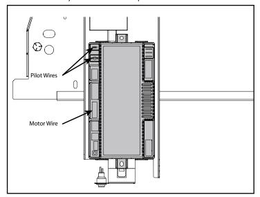
7. Disconnect the incoming gas flex line from the ball valve. Slide the pilot wires through the grommet to remove.
