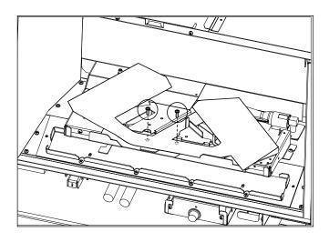
6. Remove the burner by sliding left and up out of the burner tray.
