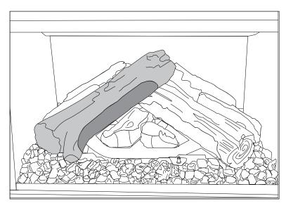
19. Place Log 8 on the pin on the front log mount. The other end will rest on the ember media.
