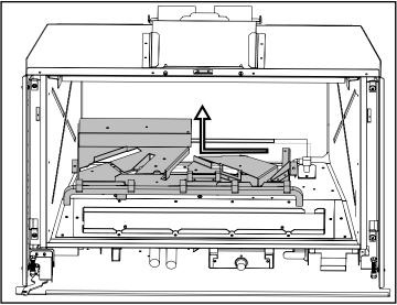
2. Remove the burner tray (2 screws).
