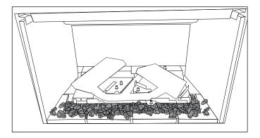
10. Fill the outside of the Burner Tray and around the Glass Tray with Black Embers as shown. Do not fill the sides of the firebox past the Burner Tray.
