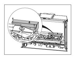
**6.** Remove the burner tray (2 screws).
