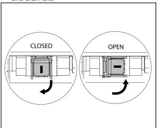
Alternatively, rotate the knob to turn it into a handle for more leverage. Clockwise closes the valve, counter-clockwise opens it.
