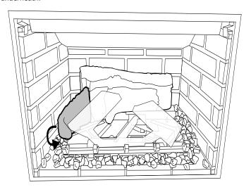
8. Place Log 3 on the pin and rotate it until it touches the tab shown below. Ensure that Log 3 is resting directly on the tray with no embers underneath.
