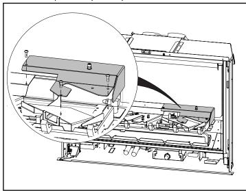
3. Slide burner tray to the left and out.
