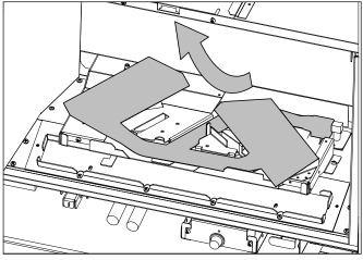
7. Install the Front Log Mount with one screw as shown.
