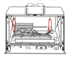
7. Slide burner tray to the left and out.
