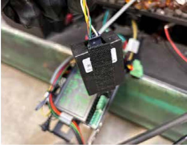
Diagram 6 Velcro affixed to WIFI dongle
