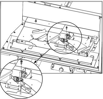
8. Re-install the burner and pilot shield.
