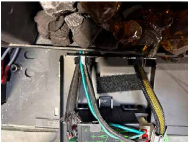
Diagram 7 Velcro affixed to IFC Tray
