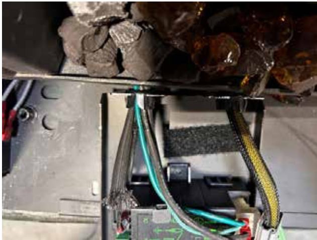
Diagram 7 Velcro affixed to IFC Tray
