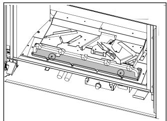
\*The front panel in the black steel/black glass panel set is a single part. The front panel for the brick panel set is split into two parts.
