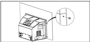
7. Slightly loosen the screws shown below on both sides.
