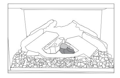
17. Place Log 6 on the right end of the burner. The log rests on the burner.
