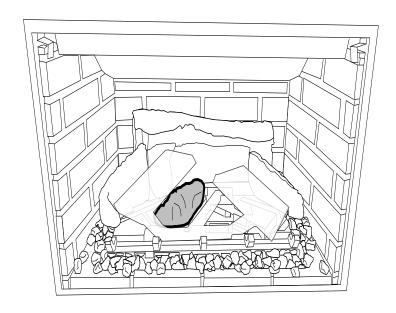
10. Place Log 5 on the pin under the right burner.
