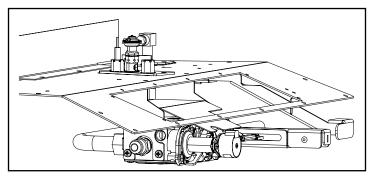
10. Reverse steps 9-1 to replace with new gas valve assembly.
