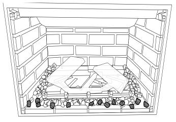
6. Carefully lay Log 1 on the two pins behind the burner. Make sure the left part of the log does not hit the left portion of the burner.
