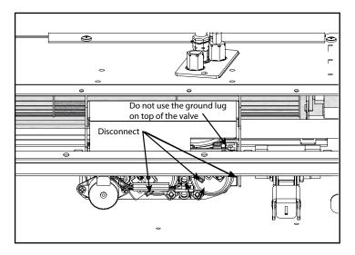
6. Slide out IFC tray and disconnect the pilot wires and motor wire.
