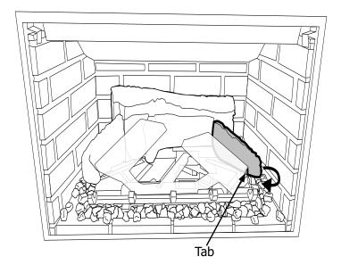
9. Place Log 4 on the two pins under the left burner.
