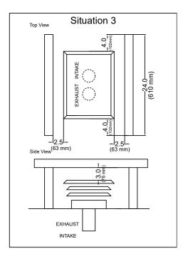
Note: Restrictor must be set to 2-1/2" (63 mm) open for NG or 4-1/2" (114 mm) open fo LP.
