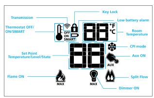
Figure 2: Transmitter LCD Display
