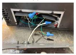
13. Tuck wires neatly into the unit using the cable ties and clip wire holder and re-install the side cover.
