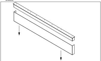
2. If using a grinder (recommended): trim the lower section to height referring to the installation table for the amount to remove.
