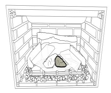
11. Place Log 6 on the grate with the notch on the middle of the log sitting on the first grate bar and the flat section pointing up. Log 6 does not sit on the front panel - it rests on the tab next to the second grate bar. Ensure that there are no embers underneath the log.
