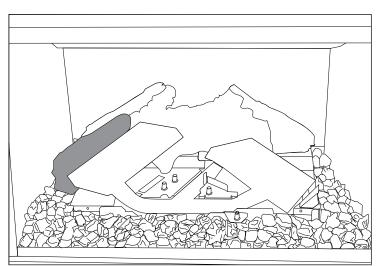
14. Place Log 3 on the pin and rotate it until it touches the tab shown below. Ensure that Log 3 is resting directly on the tray with no embers underneath.
