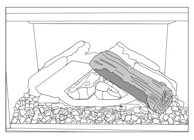
18. Place Log 7 on the left of the burner. The log rests on the burner.
