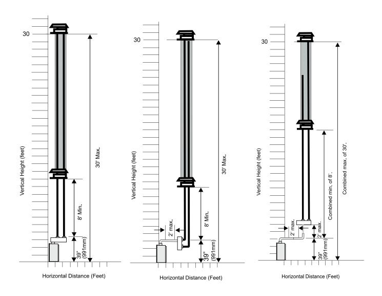
The shaded area in the diagrams show the allowable vertical terminations. Restrictor Position Set 0-3" Factory Setting  $\frac{1}{2} \left( \frac{1}{2} \right) = \frac{1}{2} \left( \frac{1}{2} \right) \left($
