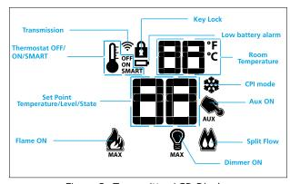
Figure 2: Transmitter LCD Display
