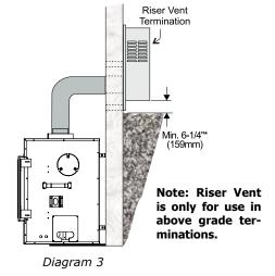
\*Diagrams 3 & 4: As specified in CSA B149.1 Installation Code. Local codes or regulations may require different clearances.
