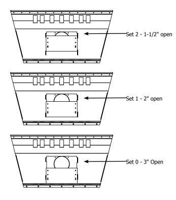
Vent restriction is required for certain venting installations, see the diagrams in the "Venting Arrangements" section to determine if they are required for your installation.
