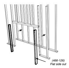
5. Secure horizontal steel header stud (466-128) with 2 screws per side as per diagram.
