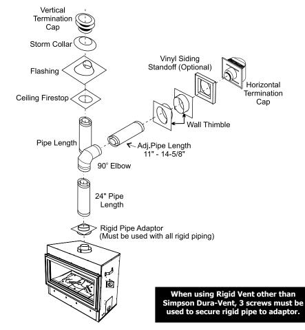
The Regency AstroCap<sup>™</sup> and Regency Riser Vent terminal are certified for installations using Regency venting systems as well as Simpson Dura-Vent® Direct Vent, American Metal Products Ameri Vent Direct Vent, Security Secure Vent®, Selkirk Direct-Temp. AstroCap<sup>™</sup> is a proprietary trademark of Regency Fireplace Products. Dura-Vent® and Direct Vent are registered and/or proprietary trademarks of Simpson Dura-Vent Co. Inc.
