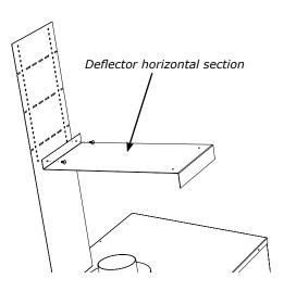
4. If the deflector extender is required, install with 2 screws, extend to desired length before tightening screws.
