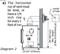
towards the termination. Never allow the vent to run downward. This could cause high temperatures and may present the possibility of a fire.
