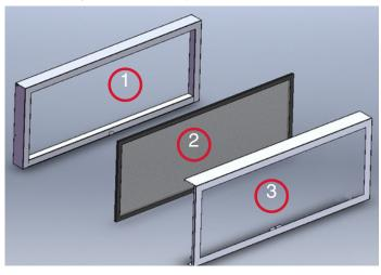
2. Remove screws from inner side of the inner door trim and discard screws and the brackets. (Brackets not shown). Remove the screen mesh from inner door trim.
