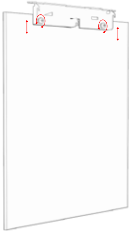
To adjust the side glass, remove the screws at the top of the panel and move the glass up or down. When the glass is in the correct position, replace and tighten the screws.
