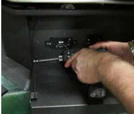
3. Remove four screws to remove the access panel (in locations shown below) and the chain attached to the front door and the unit.
