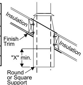
If the support extends above the roof, cut it flush with the top of the roof. Nail the support to the frame opening using (8) 3" spiral nails or #8 x 1-1/2" screws.
