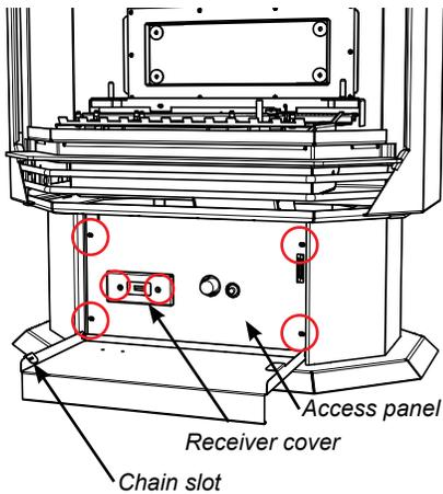
4. Disconnect receiver wire from the back of the panel and then remove panel. Set the panel on a soft cloth so it doesn't get scratched.
