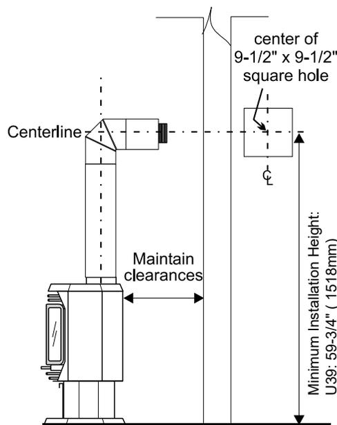
2. Assemble a **trial fit** to determine the vertical center-line for the vent termination.
