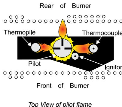
Incorrect flame pattern will have small, probably yellow flames, not coming into proper contact with the rear of the burner or thermopile.
