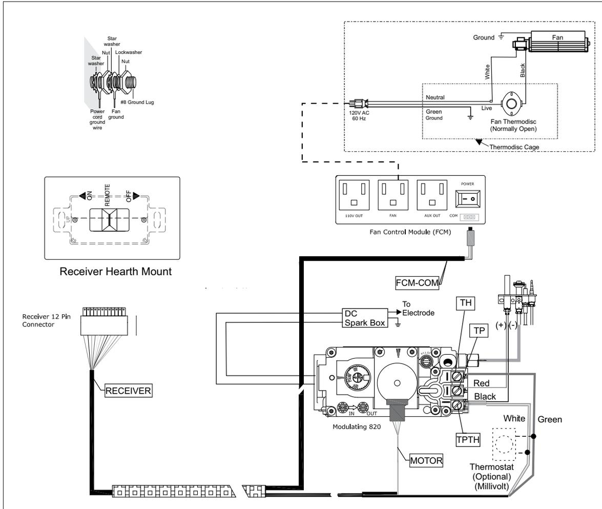
**CAUTION:** Label all wires prior to disconnection when servicing controls. Wiring errors can cause improper and dangerous operation.
