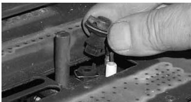
10. Unscrew the pilot orifice with the allen key and replace with the LPG pilot orifice in the kit.
