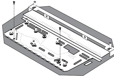
11. Remove all 18 screws holding the burner tray assembly in place.
