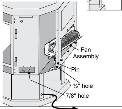
5. Lift fan off of the 2 pins, tip back and pull through firebox opening. Disconnect the green ground wire from the right side of the fan as soon as you can reach it.
