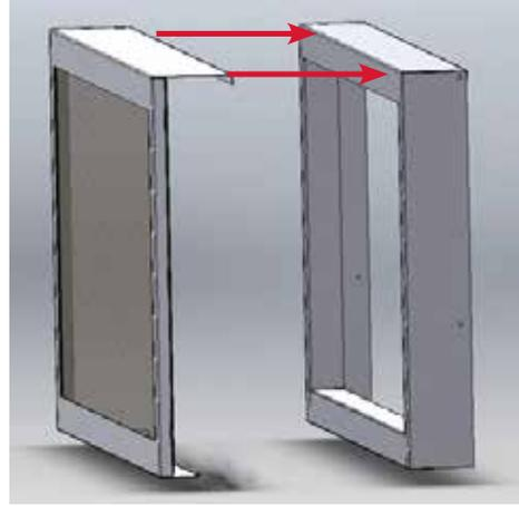
5. Bend the center tab up and secure with a screw to attach the inner door frame/safety screen assembly to the inner door trim.
