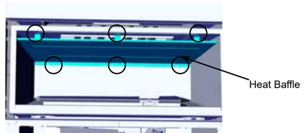
3. Remove the screws that hold the vent restrictor in place.
