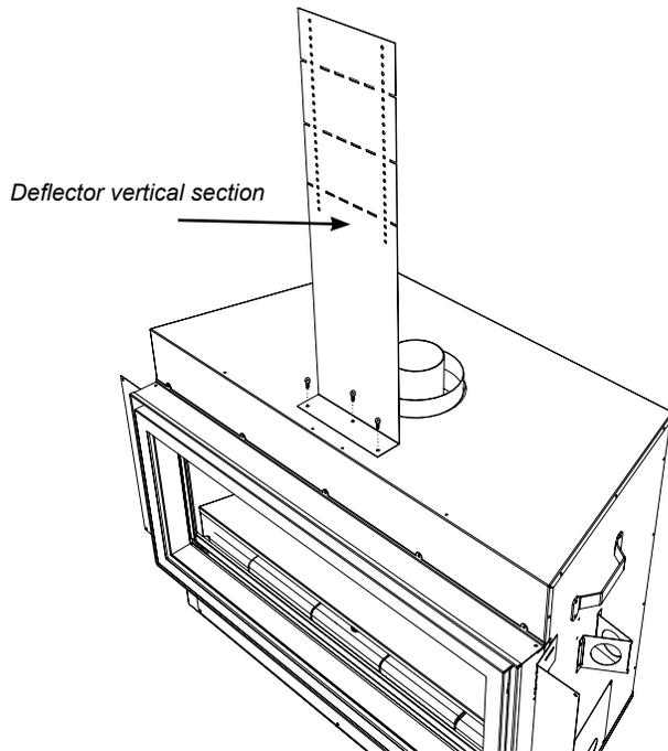
3. Install the horizontal section of the deflector to the vertical section at the desired height with 2 screws.
