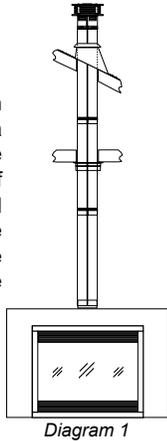
2. Set the gas appliance in its desired location. Drop a plumb bob down from the ceiling to the position of the appliance flue exit, and mark the location where the vent will penetrate the ceiling. Drill a small hole at this point. Next, drop a plumb bob from the roof to the hole previously drilled in the ceiling, and mark the spot where the vent will penetrate the roof.
