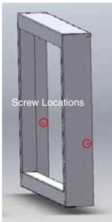
3. Install screen into inner door frame - secure safety screen by bending in 6 tabs in locations shown below.
