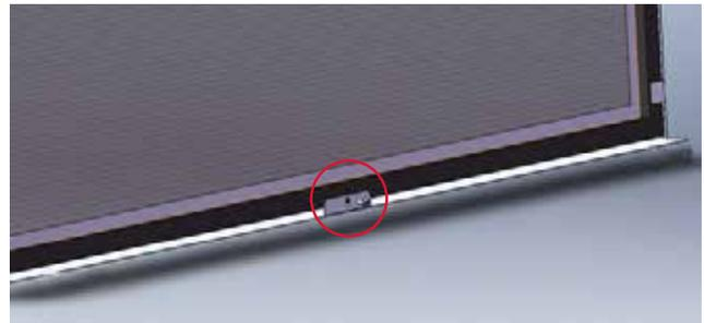
6. Bend in magnetic tabs—located in lower corners of the frame (lower left shown below).
