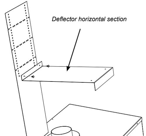
4. If the deflector extender is required, install with 2 screws, extend to desired length before tightening screws.
