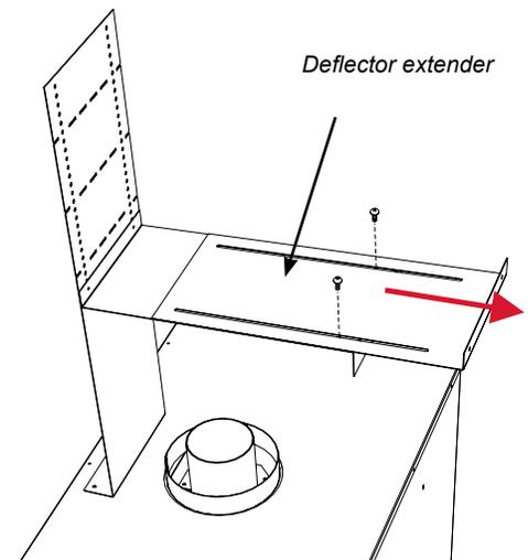
5. If there is any excess material on the horizontal section of the deflector, it can be folded down at the fold lines.
