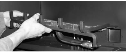
Diagram 1: Remove the left and right screws and then lift out the burner/grate assembly.
