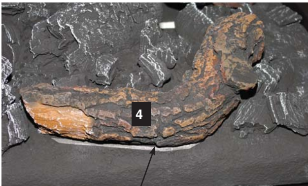
Ridge in burner tray (highlighted)
