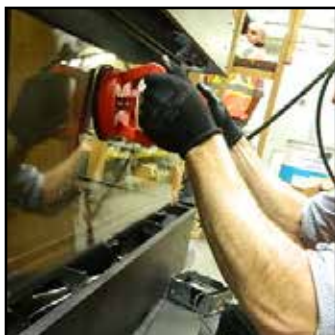
Handle glass with supplied vacuum clamps
